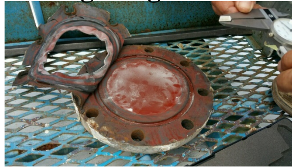
O-ring groove on blank flange. Note: A gasket was used with an unknown sealant.
