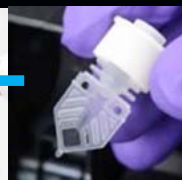
Reaction tube containing lyophilized chemical assay bead (proprietary)
