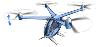
Figure 3. Concept aircraft: single-passenger quadrotor with electric propulsion.
