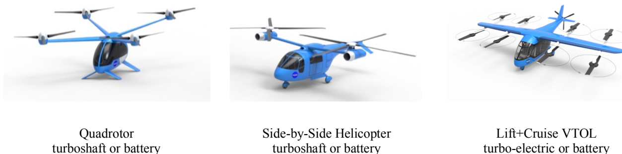
Figure 7. UAM aircraft designs: six occupants (1200 lb), 75 nm range.
