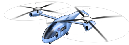
Figure 3. Concept aircraft: single-passenger quadrotor with electric propulsion.
