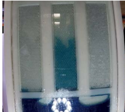
Figure 11. b) Super omniphobic coating apparatus while in zero gravity with air bubble in the reservoir on the right side.
