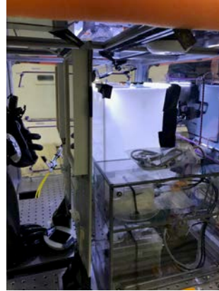
Figure 10. b) Interior of glove port box with all experiments, lights, and GoPros mounted
