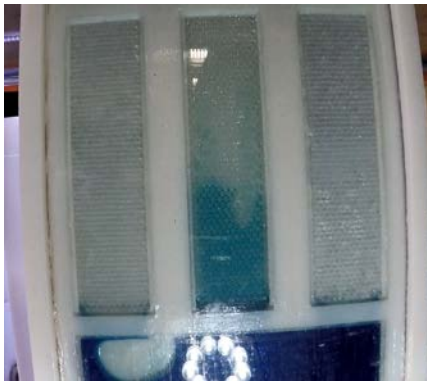
Figure 11. a) Super omniphobic coating apparatus while in zero gravity with air bubble in the reservoir on the left side.
