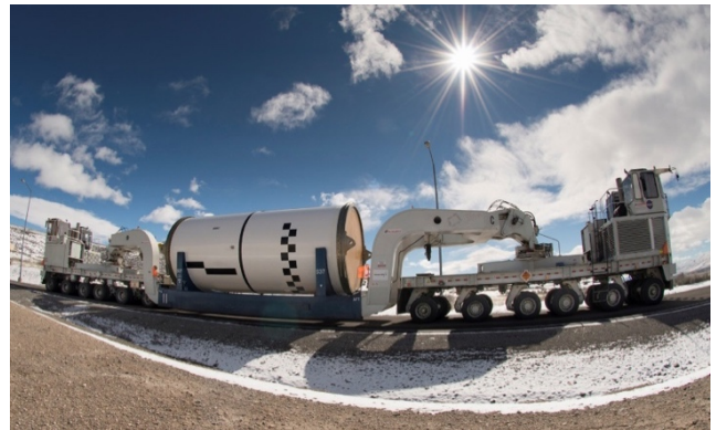
Fig. 10. Northrop Grumman has nearly completed the five-segment solid rocket boosters for EM-1; motor segments will be shipped to Kennedy Space Center, where they will be stacked to assemble the final boosters.
