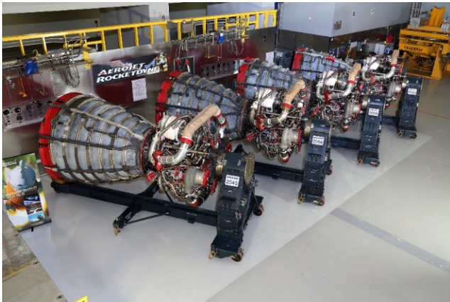
Fig. 9. All four EM-1 RS-25 engines have been tested and verified; they are ready for integration into the core stage and flight.
