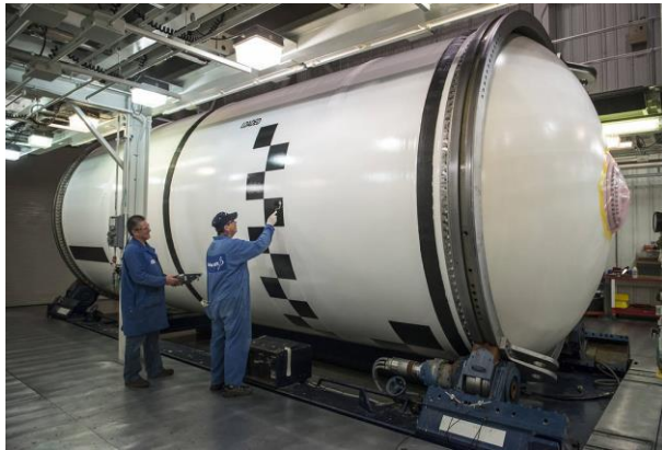
Fig. 9. Technicians apply tracking markings to an EM-1 booster motor segment at Northrop Grumman
