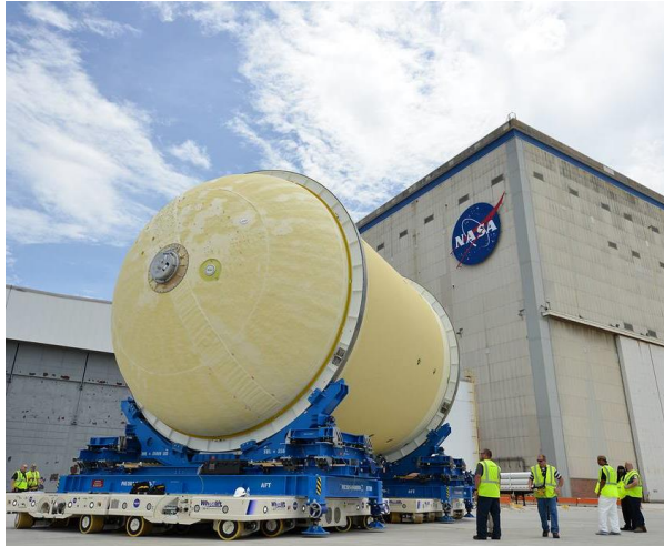
Fig. 7. EM-1 LOX tank with TPS applied
