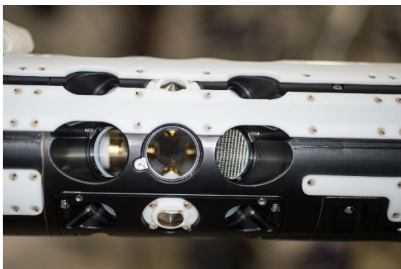
The Electrostatic Levitation Furnace (ELF) sample cartridge. Photo Credit: NASA
