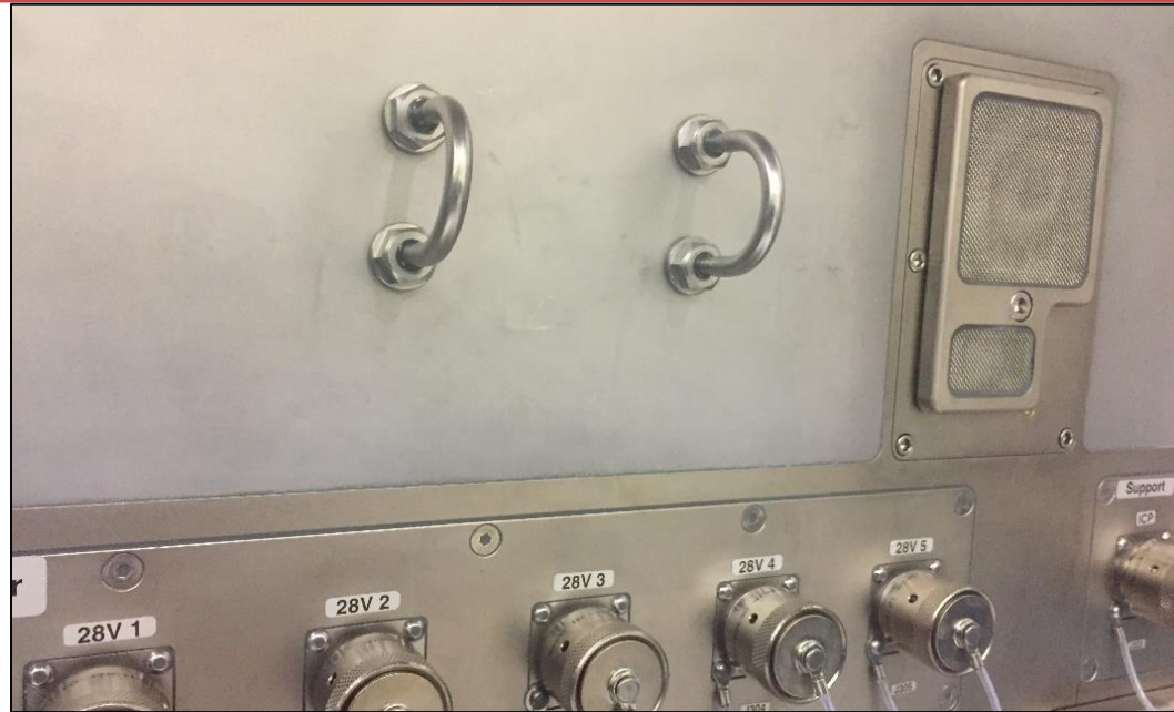
Two Cable Mounts shown attached to the ferrous surface of the LSG WV back wall.
