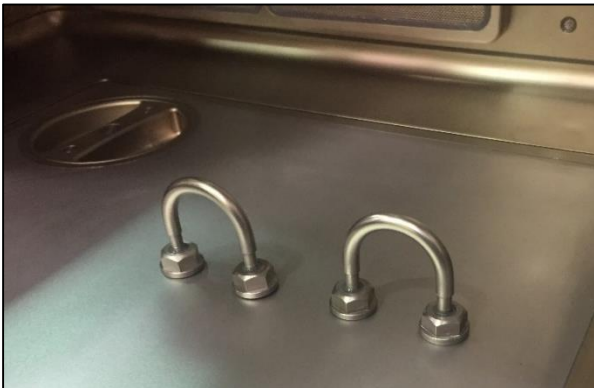
Two Cable Mounts shown attached to the ferrous floor panels.
