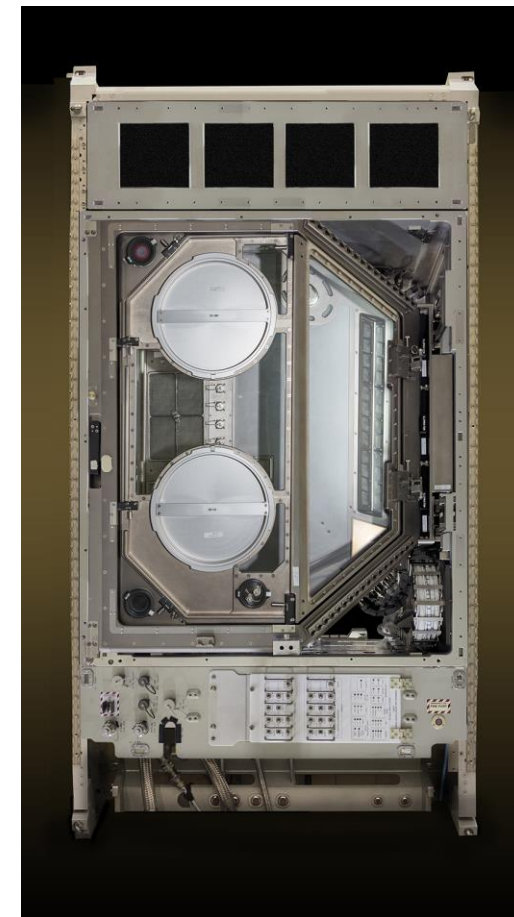
LSG with Work Volume (WV) retracted
