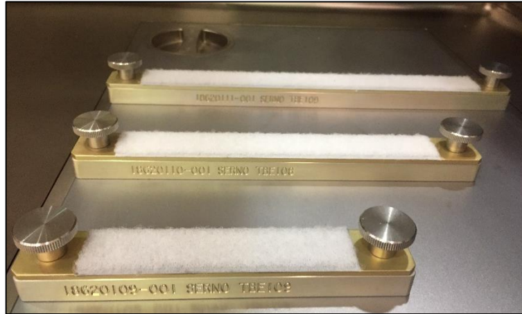
Three sizes of Magnetic Adapters with Velcro Strips: 6", 9", & 12"
