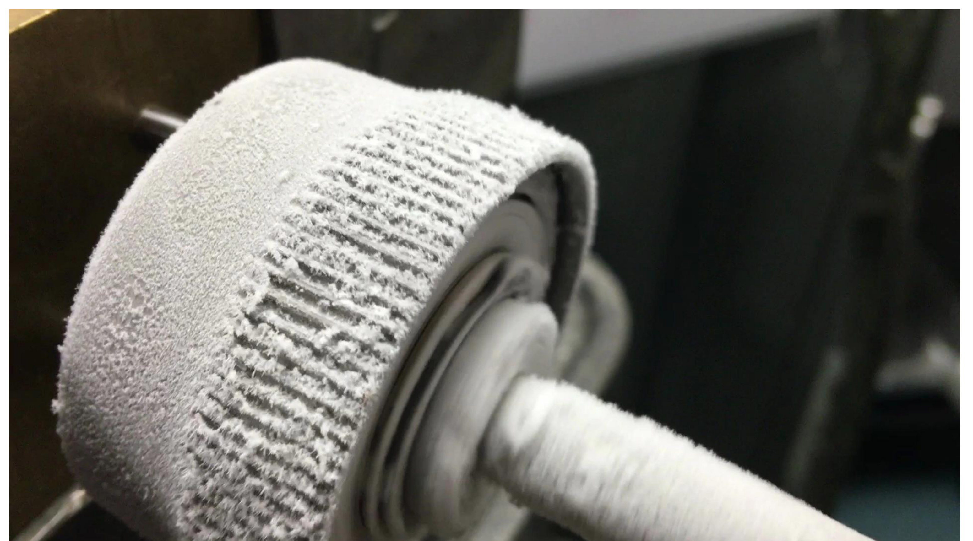
A bulk metallic glass (BMG) gear during cryogenic testing by NASA.
