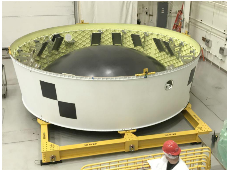
Figure 12. The Orion Stage Adapter (OSA), prior to shipping to Kennedy Space Center (KSC), showing the mounting brackets for the secondary payload dispensers and avionics unit
