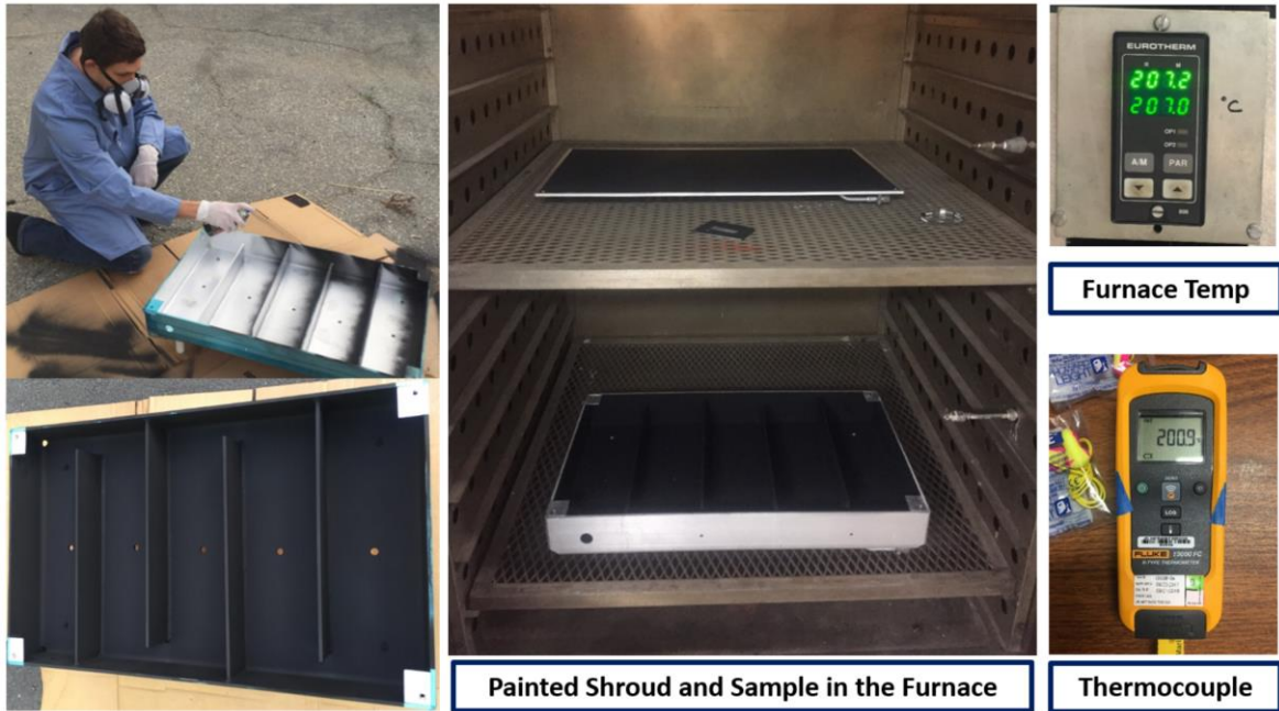
Figure 7.1.2.1-8. Shroud Spray Painting and Bake-out
