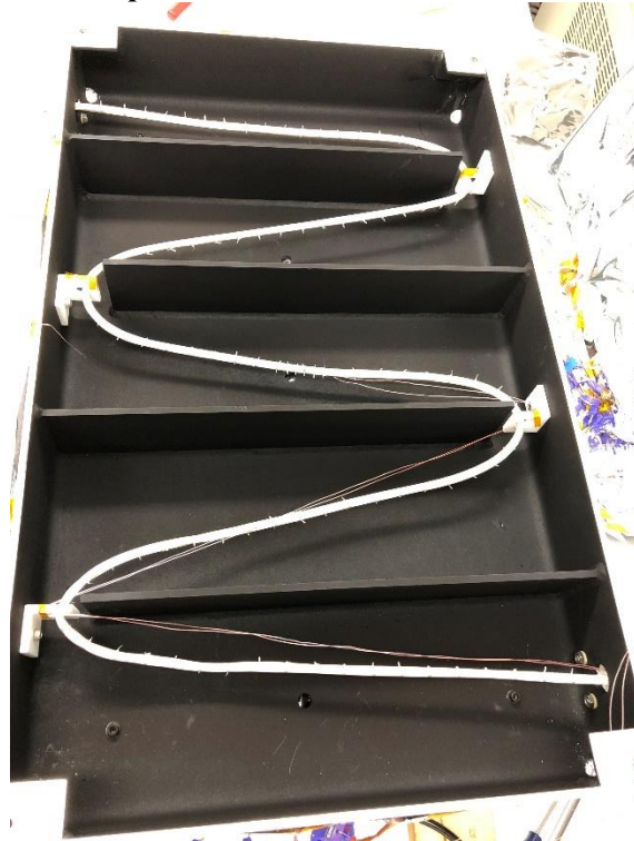
Figure 7.1.2.1-2. Interior of the Temperature-Controlled Shroud with a Wire Bundle Installed
