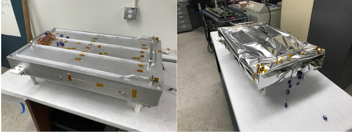
Figure 7.1.2.1-1. Temperature-Controlled Shroud with Thermocouples
