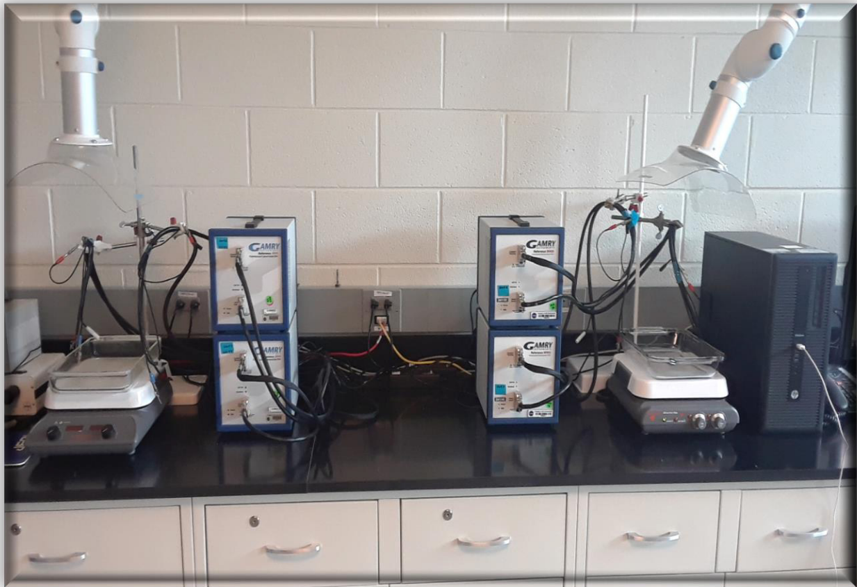
Figure 2a: Typical workstation and test cell configuration showing four Gamry 3000 ready for use.
