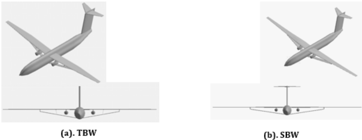
Figure 8. Minimum Fuel Weight configurations for TBW and SBW at Mach= 0.70.
