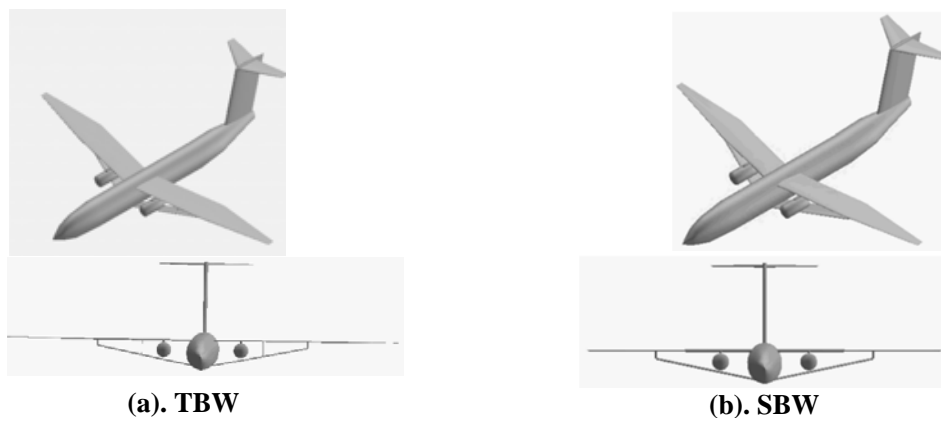
Figure 11. Minimum Fuel Weight configurations for TBW at Mach= 0.80.
