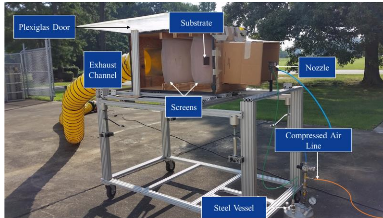
Figure 5. Labeled image of the contamination rig utilized to evaluate PSL surface contamination.
