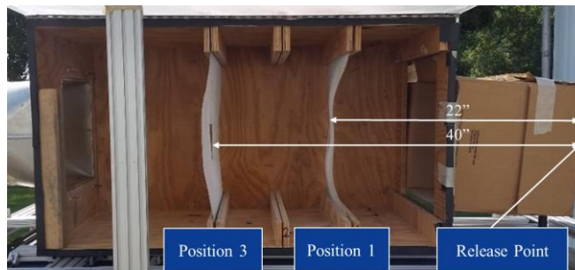
Figure 8. Position of screen coupons for contamination testing.
