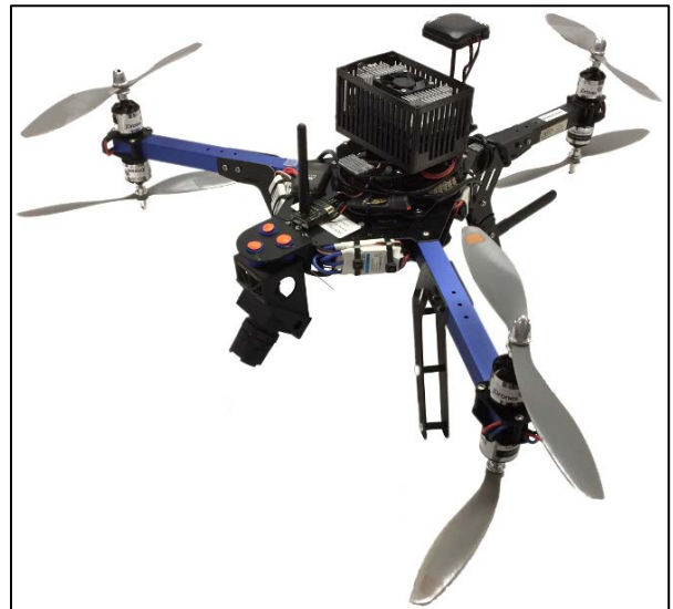
Figure 2- 3DR Y-6 research vehicle with research computer and camera installed.
