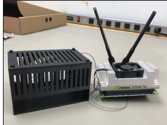
Figure 4 - Jetson TX-2 research computer along with 3D printed enclosure and WiFi antennas.
