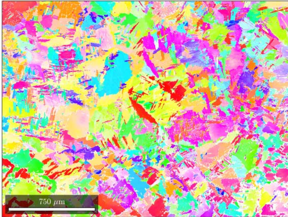
Figure 5. An inverse pole figure (IPF) map of the highly twinned microstructure of the Ti-8Al-1Er alloy. The twins are compression twins with a misorientation of 57-64 degrees.
