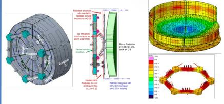
Design of 'zonal' rear heater system to actively control mirror system thermal environment
