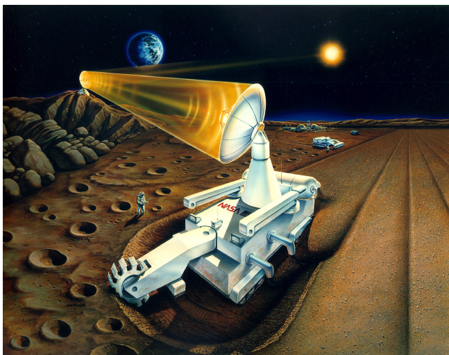
Figure 29.—Automated Mark II lunar miner for extracting He-3 and solar-wind-implanted volatiles from Moon regolith. Courtesy of J. Andrews, Fusion Technology Institute, University of Wisconsin-Madison.
