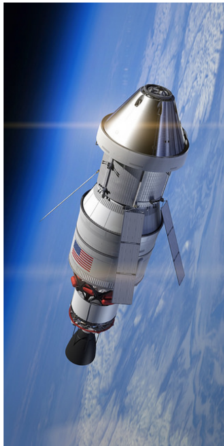
Figure 11. Orion with ICPS (missions EM-1 and EM-2)
