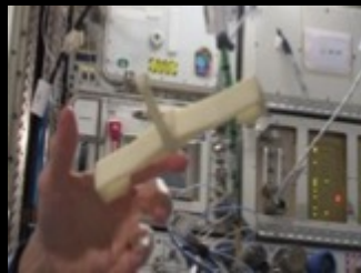
SPHERES Tow Hitch: SPHERES consists of 3 free-flying satellites on-board the ISS. Tow hitch joins two of the SPHERES satellites together during flight. Printed 2/21/17.
