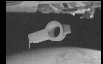
OGS Adapter: Adapter attaches over the OGS air outlet and fixtures the velocicalc probe in the optimal location to obtain a consistent and accurate reading of airflow through the port. 7/19/2016.
