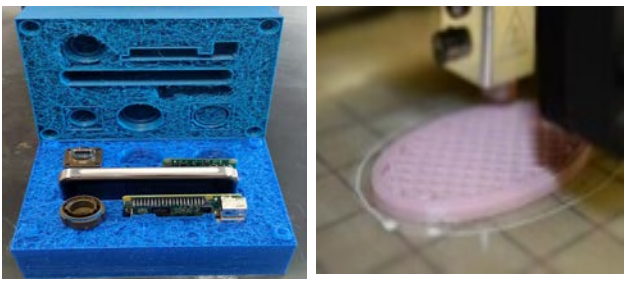
TU Recyclable Launch Container (Left); CRG Printed Part from Recycled Baggie (Right)
