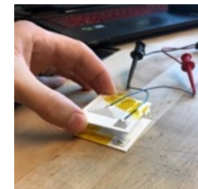
Printed Wireless Humidity Sensor
