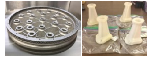
Design Database Development Printed Life Support System (LSS) Retaining Plate (Left); Urine Funnels (Right)
