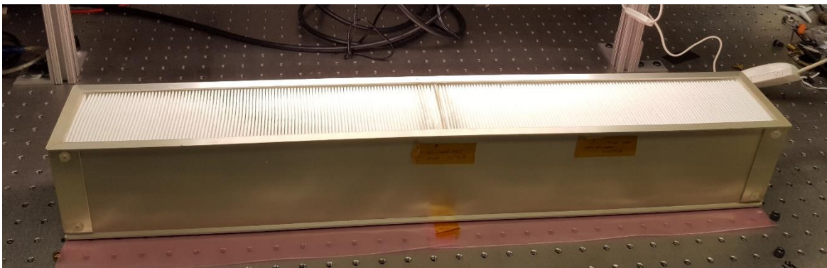
Figure 1: ISS Bacteria Filter Element (BFE) with Nomex ® inlet screen removed.
