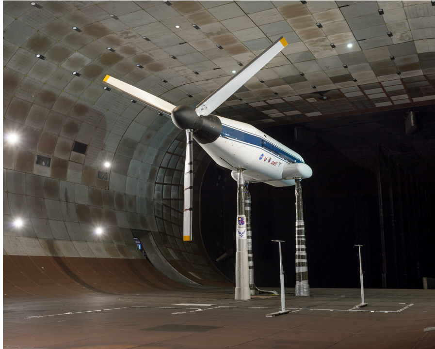
Fig. 1. TTR/609 installed in the USAF National Full-Scale Aerodynamics Complex (NFAC) 40x80-foot test section.
