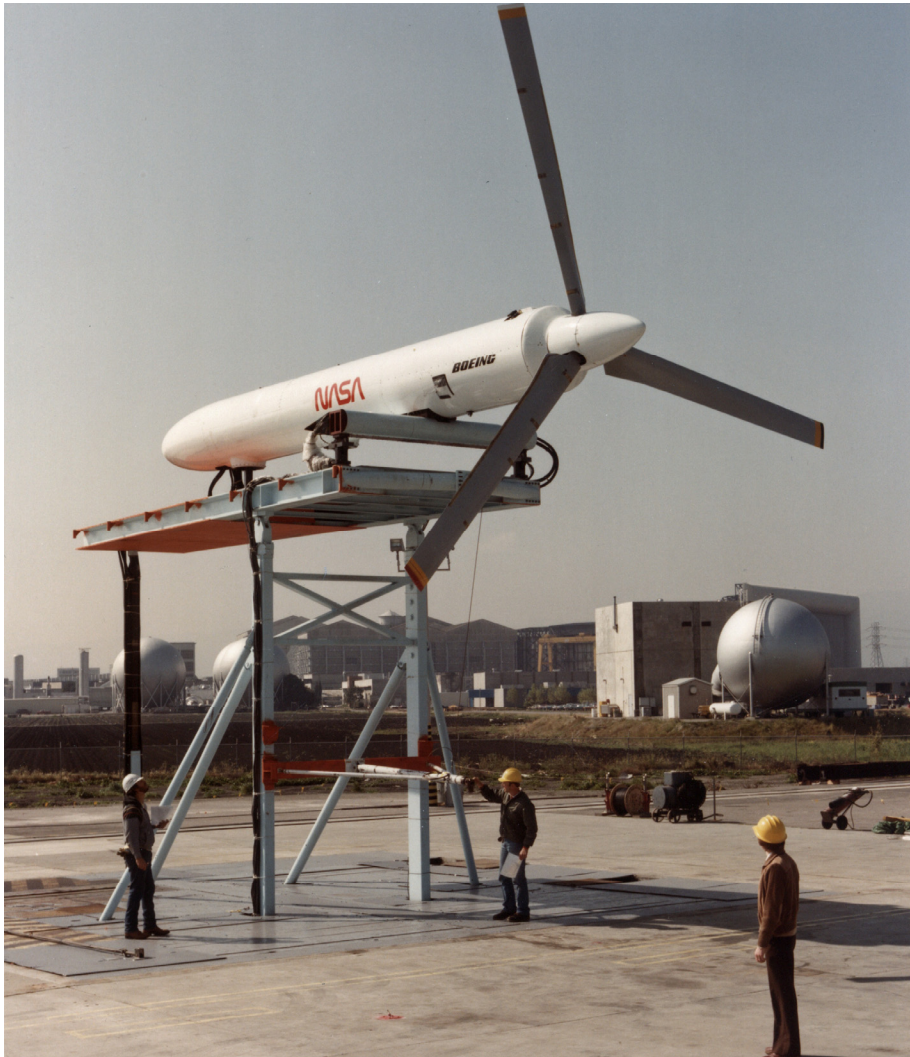
Fig. 2. XV-15 metal-bladed proprotor tested in hover at the NASA OARF in March of 1984 and 217 thrust–power data points obtained.
