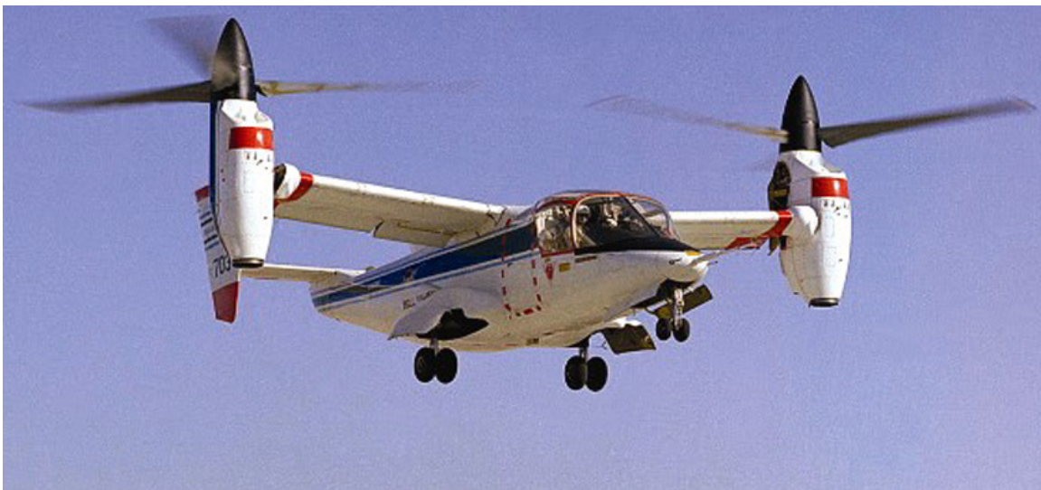
Fig. 11. The world’s first successful tiltrotor VTOL was the XV-15. This experimental aircraft was championed by NASA and the U.S. Army and developed by Bell Helicopter Textron.
