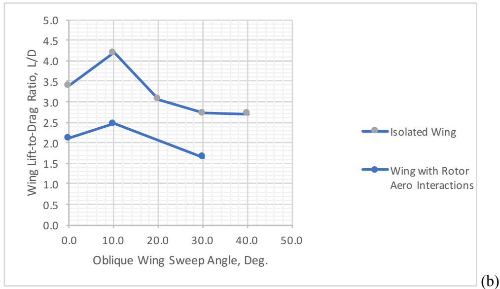
Figure 12. Influence of the wing oblique sweep angle on cruise L/D
