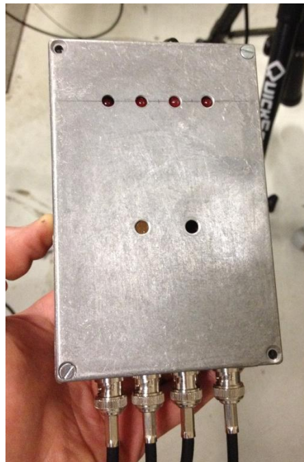
Figure 38 - Four LED timed light sequencer, horizontal spacing is 15.2 mm.
