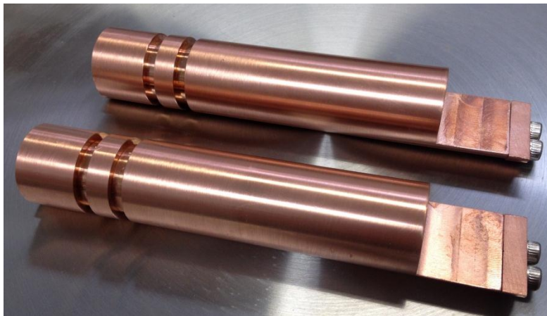
Figure 33 - Machined copper conductors showing double seal O-ring grooves.
