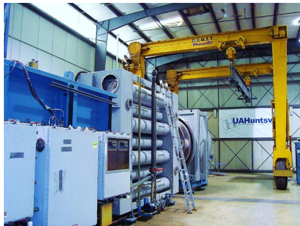
Figure 47 - The Charger 1 Pulse Power Research Facility provides 3 TW and 572 kJ of electrical energy into pinch loads.
