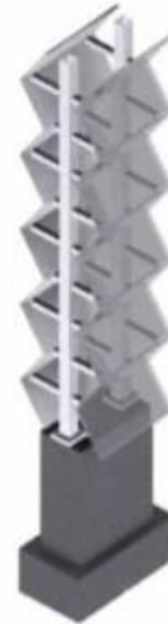
Figure 4.2. Prototype of a 3D PV. 3D mixed mirrors and solar cell structure optimize the conversion from a specific volume.
