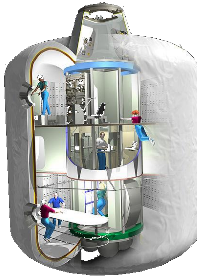
Figure 12. NASA Reference TransHab Design (credit: NASA)
