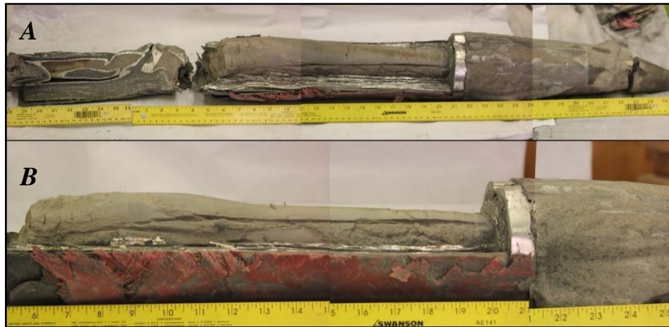
Figure 50. (A) The core sample was exposed after removing the encasing material; (B) note the swelling in the sample diameter near the aft end of the core, indicative of increasing pressures occurring forward of the section that experienced severe deformation.
