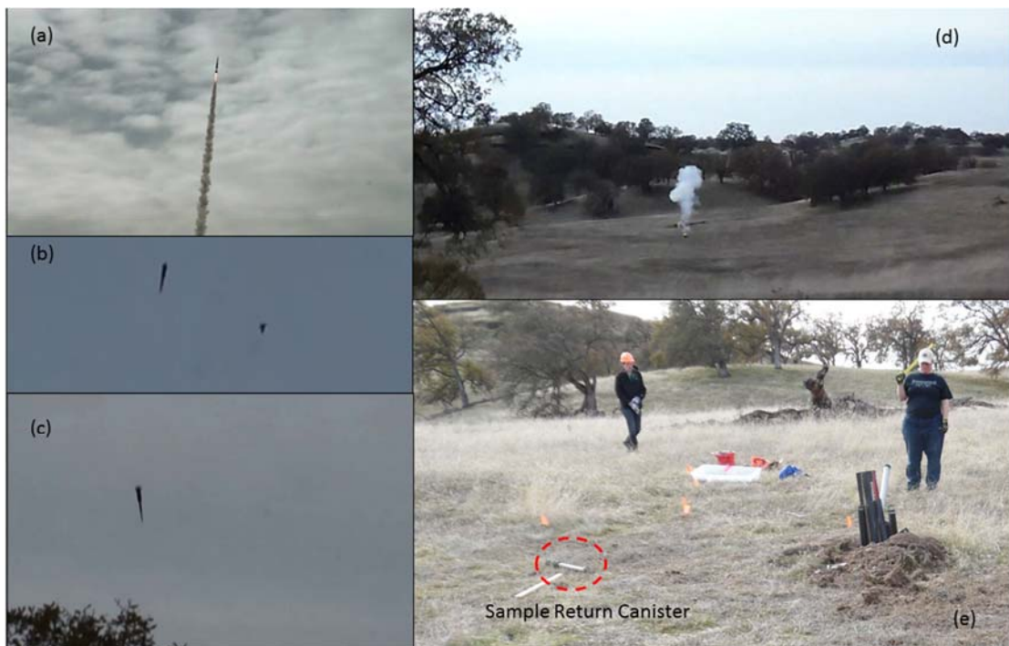
Figure 52. (a) Launch of the 3 rd generation penetrator, (b) separation of booster and penetrator shortly after apogee (c) the penetrator at Mach 1 just above tree height, (d) impact and (e) close-up of the impact site showing the SRC ejected about 2 m from the impact sight.
