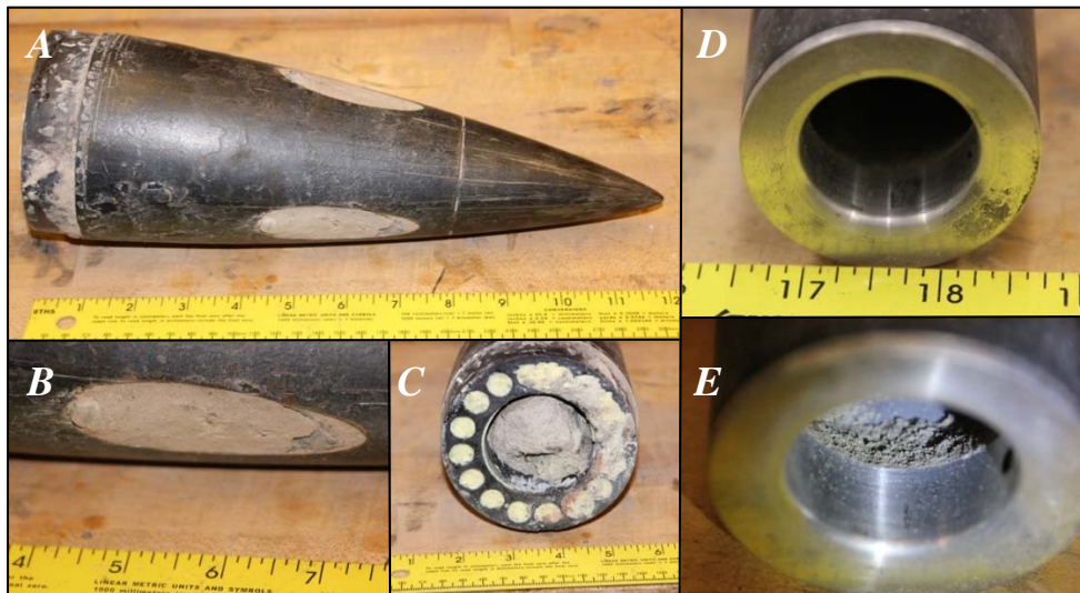
Figure 40. (A) The nose cone experienced no deformation during impact, (B) and feed ports opened successfully. (C) Ejecta experienced stagnation at the start of the feed chimney; (D) the backflow baffle inside the SRC successfully collected fine ejecta (E) that traveled through the feed chimney.
