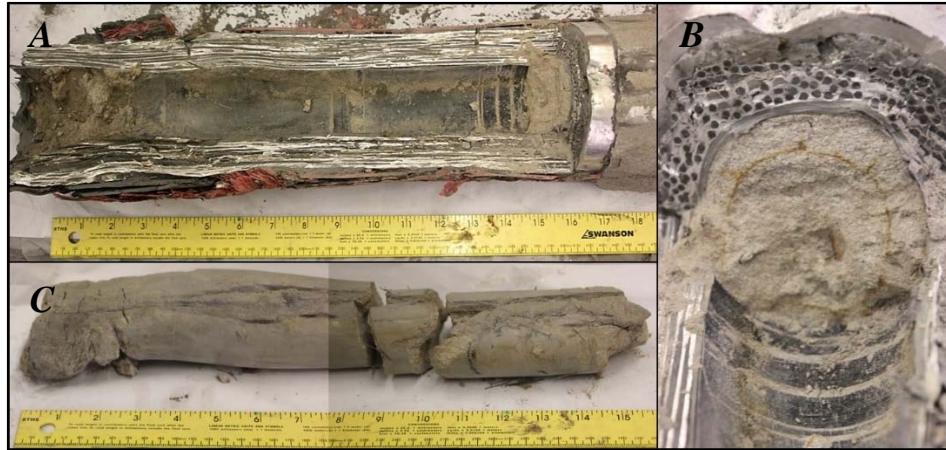
Figure 51. (A) The feed chimney after the removal of the core sample; (B) the sample core was very solid, and required fracturing it in multiple locations to remove it from the chimney; (C) sample material in the nose cone was left in place given the difficulty in removing it intact.
