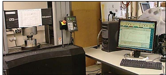
Figure 20. The Instron 5585H Series Floor Model Testing System used for compression testing [Winglee et al, 2013].
