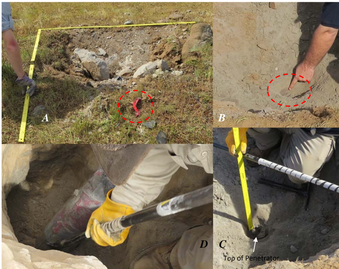
Figure 45. (A) The surface of the impact site exhibited a limited ejecta fan (less than 1.8 X 1.8 meters), with some material overturn, and fracturing of the sandstone around the impact shaft isolated to the top few inches near the surface, the SRC attachment bracket was found above the surface (red circle); (B) backfill debris filling the 4 inch diameter impact shaft highlighted by the red circle; (C) once backfill was removed, slickensides indicative of penetrator embedding aligned along the impacting vector; (D) recovery crews spent more than ten hours removing blocks of sandstone with hand tools, excavating to a depth of 1.6 meters.
