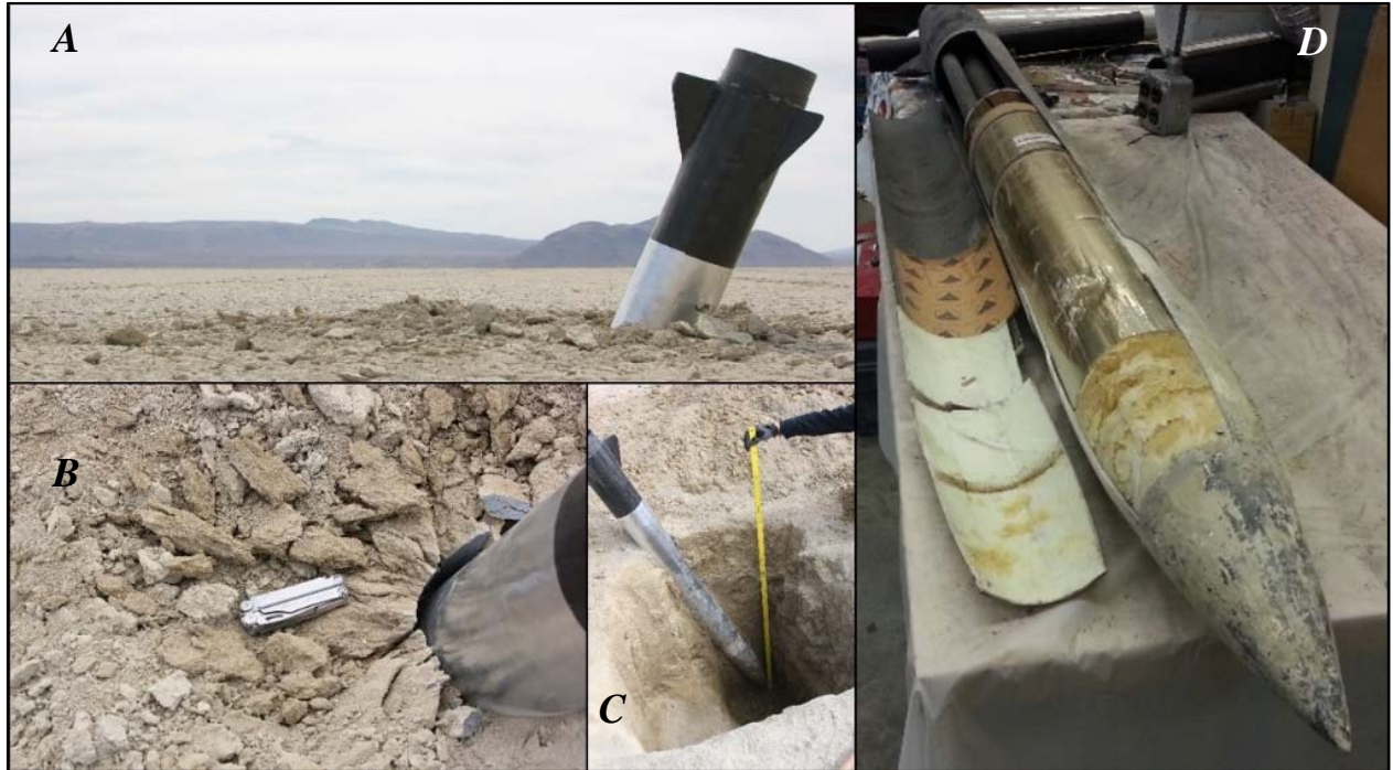
Figure 31. (A) During the flight of Gravedigger 1, the second stage motor casing failed during ignition when the forward enclosure sheared off. While the penetrator was blown clear, the resulting impact velocity was lower than desired ( \sim 180 m/s). (B) The impact created a clearly defined crater, with radial fractures in the playa, (C) and the penetrator embedded to a depth of 1.32 meters at an angle of \sim 30^\circ off normal. (D) Post recovery examination of Gravedigger 1 revealed the impact resulted in almost no internal damage to the penetrator, but the impact velocity was too low to open the feed ports that had been covered with carbon fiber, so no sample was collected.
