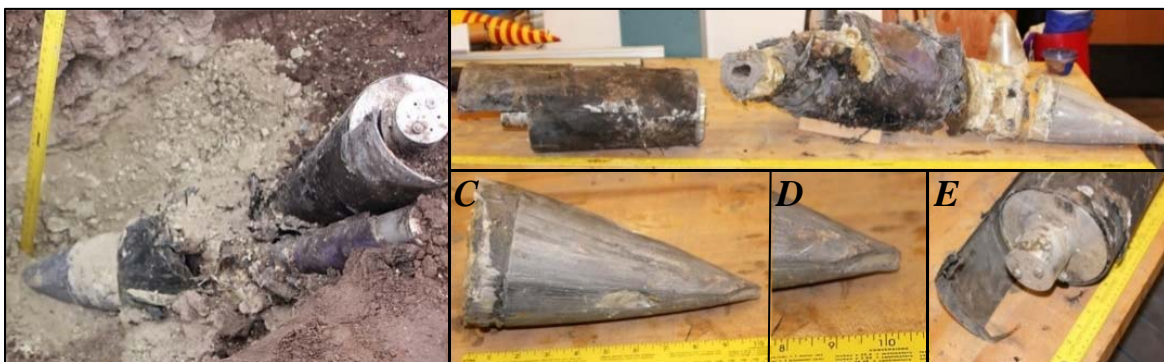
Figure 42. (A) The penetrator embedded to a depth of \sim 0.9 meters, but was deflected off a straight trajectory when it struck a piece of quartzite; (B) the deflection resulted in massive deformation of the penetrator that separated the body at unreinforced seams in the energy absorbing core material, and prevented sample material from reaching the SRC; (C) the aluminum nose cone experienced some deformation during the impact, although the feed ports remained open; (D) the contact point where the nose cone encountered the quartzite; (E) the SRC remained intact, but warping in the airframe resulted in binding.
