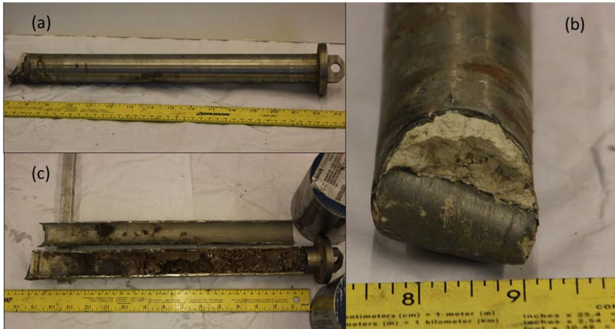
Figure 53. (a) Sample return canister after recovery, (b) the end of the canister showing partial self-sealing of the sample and (c) cutaway of the canister showing the captured sample including its stratigraphy.
