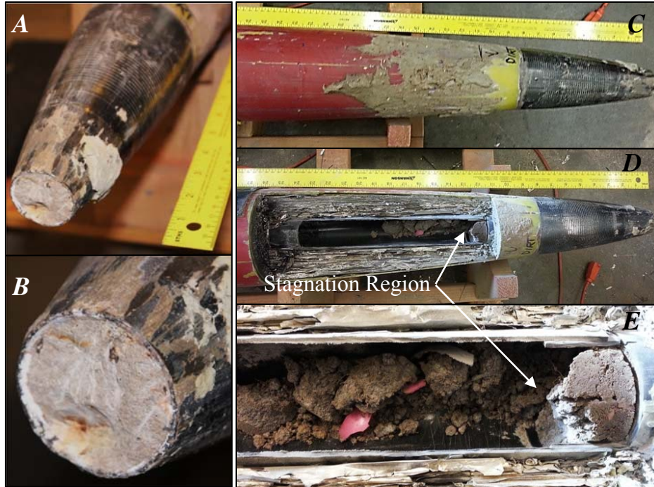
Figure 38. (A & B) The center-bored feed port, steel nose cone sustained no significant damage; (C) measurements made through the aft of the penetrator suggested material flow had stagnated around 0.33 meters after impact; (D) the penetrator in cross-section, showing the stagnated material inside the feed chimney; (E) close-up of the stagnation point with remnants of the feed port cover (pink shell fragments) mixed in the ejecta.
