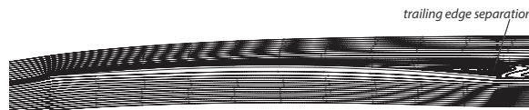
Figure 21. Streamlines for the cambered plate showing trailing edge separation ( \alpha = 8.0^\circ , M = 0.20 , Re \approx 2.0 \cdot 10^3 )
