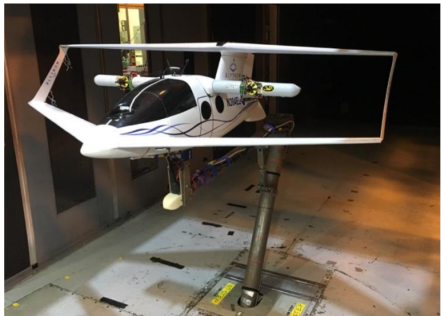
Figure 15. Elytron 4S UAV installed in the U.S. Army 7- by 10-Foot Wind Tunnel.
