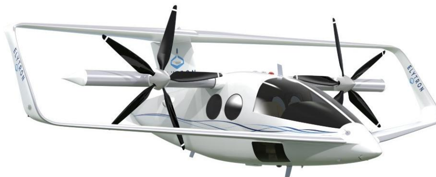
Figure 1. CAD rendering of Elytron 4S (full-scale) conceptual design.
