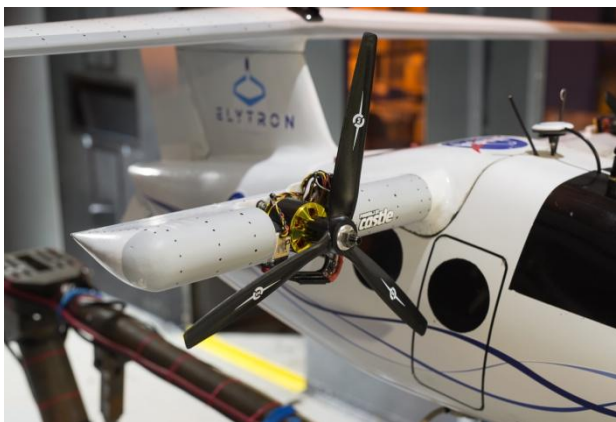
Figure 3. Close-up of Elytron 4S UAV protruding antennae, motor cutout, tuft (dots), and exposed cabling.
