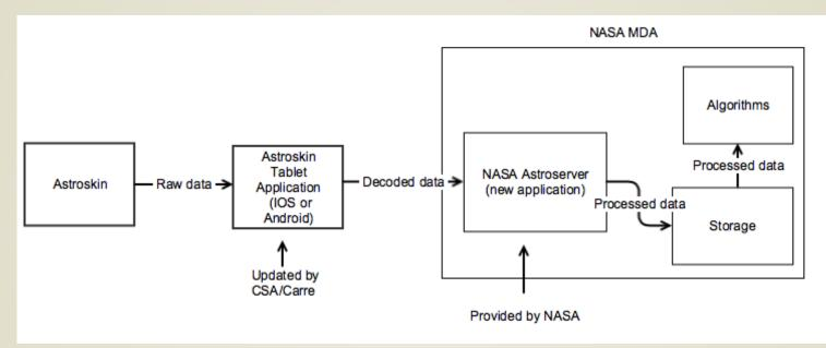
MDA system integration tests with the Astroskin scheduled for FY17
