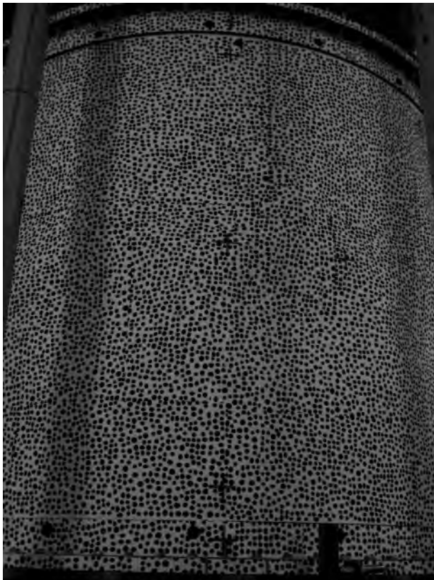
FIGURE 1. Measurement of structural deformation of a large cylinder during failure. Original image (left) compared with the Motion Magnification of the image (right).
