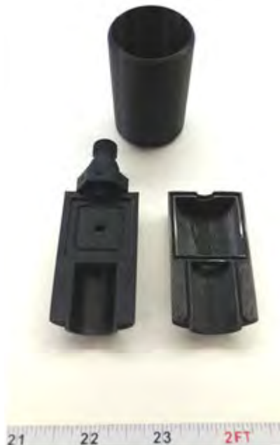
FIGURE 4. 3D-printed ECLSS pressure switch housing in ULTEM.
