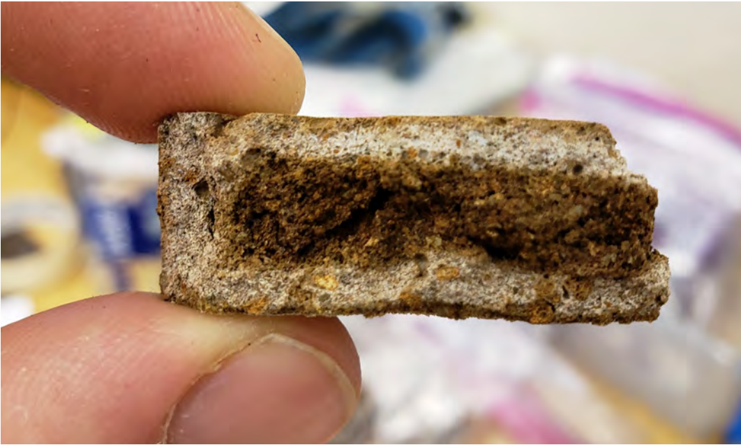
FIGURE 3: Sodium silicate and Martian simulant mixture cured in CO 2 . Note the formation of a sodium bicarbonate rind.
