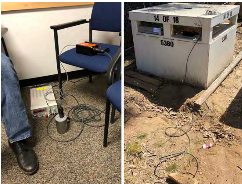
FIGURE 3. Commercial sensor (left) and field set-up (right). The seismometer is buried under the rock in the foreground.
