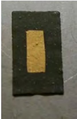
FIGURE 3. Composite pressure/temperature sensor for ECLSS materials developed by ISM.
