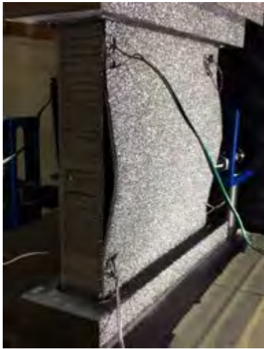
FIGURE 2. Predictive failure analysis (PFA) of a hoop edgewise compressions (HEWC) coupon and a failed HEWC coupon. Pretest predictions were within 9% of testing results.
