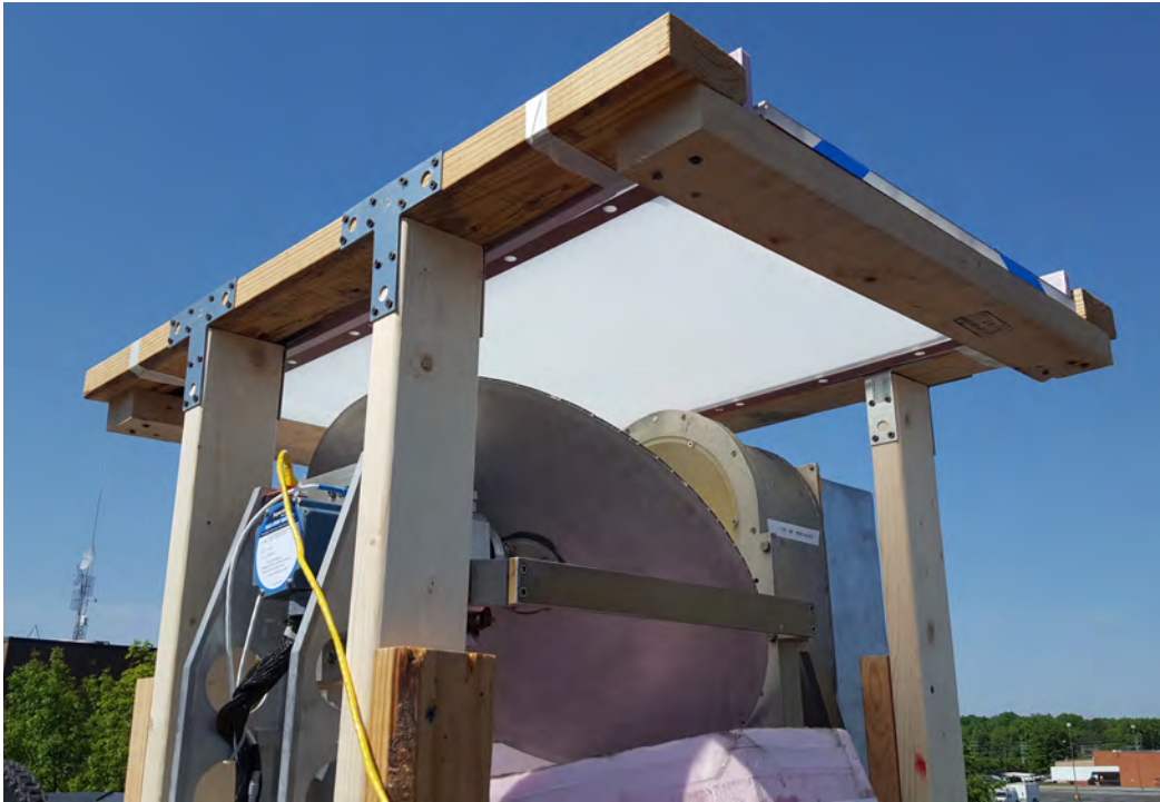
FIGURE 2. AMPR sky test using the new radome. The instrument is rotated 180° to point skyward, and the wood mounting holds the radome above it at a distance equal to that experienced in the NASA P-3 bomb bay mounting. Sky tests enable calculation of the transmission coefficients for each channel/frequency.
