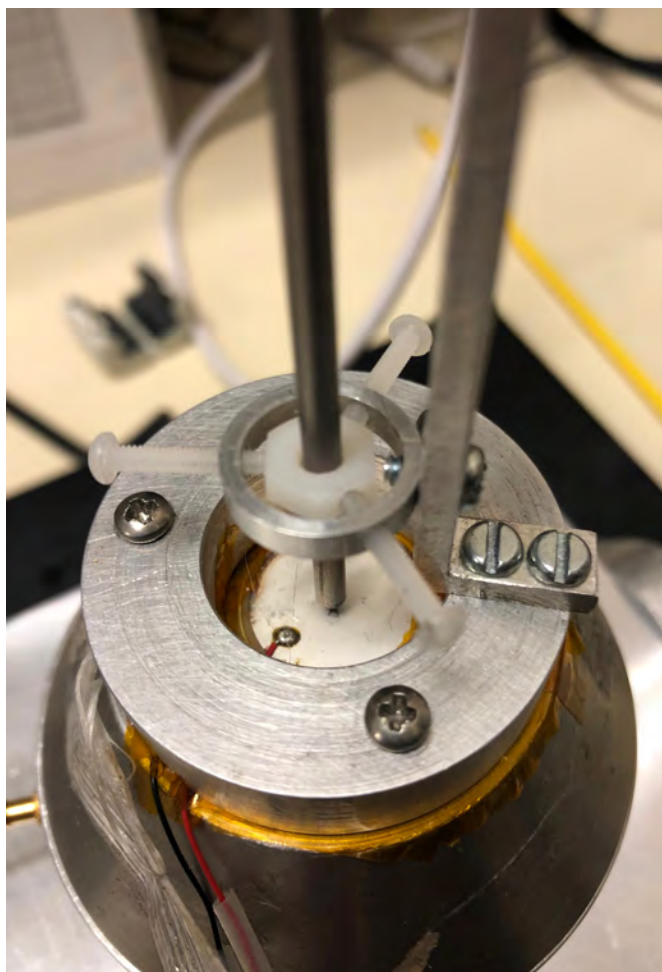
FIGURE 1. Piezo sensor mounted in test assembly.
