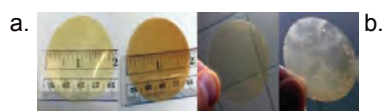
FIGURE 1. Photographs of the first-generation ionic polyimide films: (a) neat and with \approx 25 wt% 'free' [\text{C}_2\text{mim}][\text{Tf}_2\text{N}] content and (b) the difference in optical clarity when 'free' IL is present illustrated.
