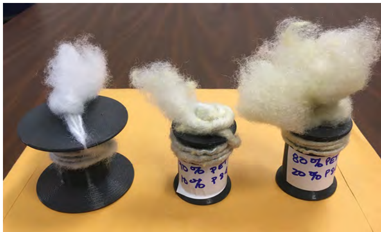
FIGURE 4. Carded and spun yarns containing 100% PET (left), 90% PET/10% P84 (center), and 80% PET/20% P84 (right).
