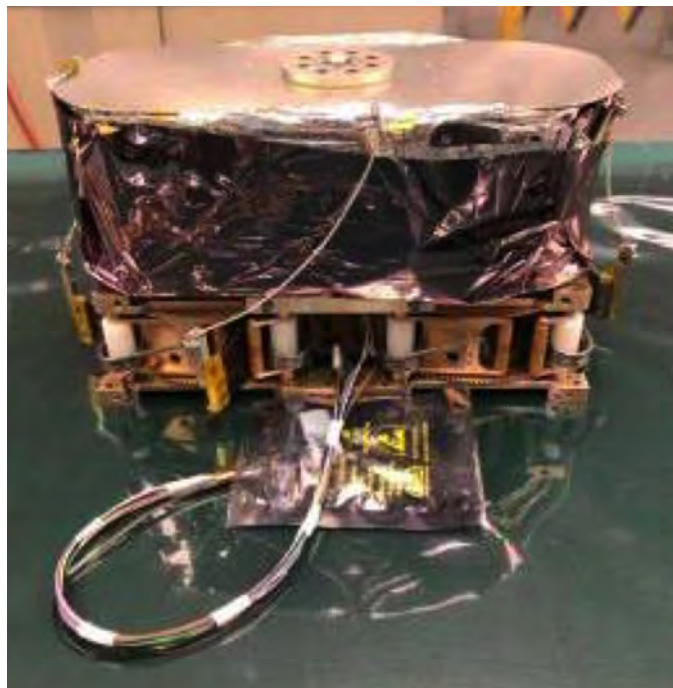
FIGURE 1. The NEA Scout solar sail and booms integrated into the deployment system before deployment.
