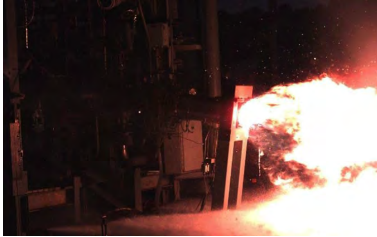
FIGURE 2. Combustion test article hot fire.
