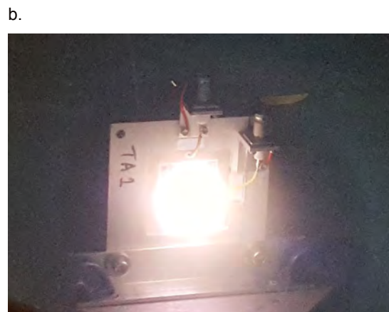
FIGURE 1. Photograph of the LTCC-ET (a) packaged for testing and (b) during a plasma ignition test with Argon gas.
