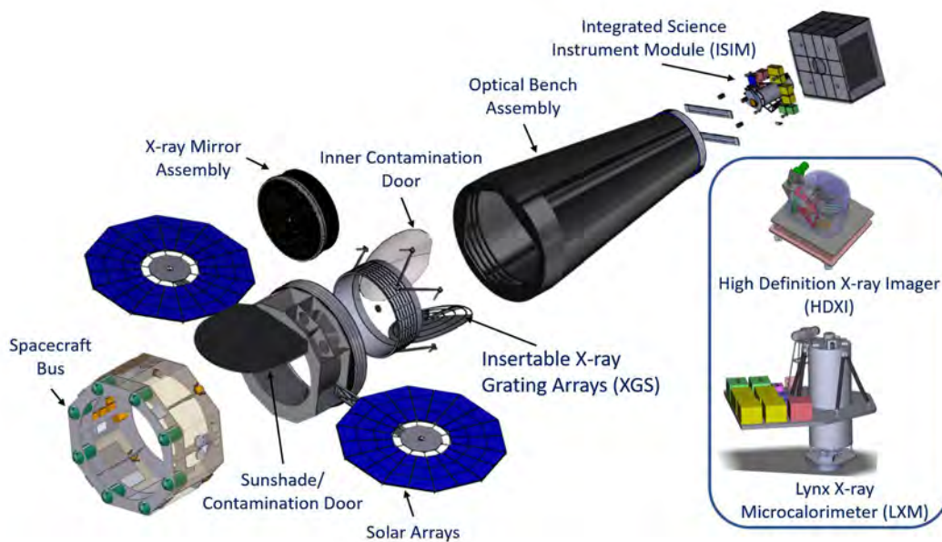
FIGURE 2. Lynx has a 10-m focal length and consists of a high-resolution, 3-meter diameter, large area X-ray mirror assembly with pre- and post-collimators (XMA) surrounded by the spacecraft bus and complemented by an instrument suite that includes a low-noise megapixel imaging array (HDXI); a large-format, high-spectral-resolution, small-pixel array (LXM), and high-efficiency, high-spectral-resolution, dispersive spectrometer (XGS). Detectors for all three instruments are mounted onto the ISIM.
