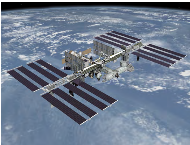
FIGURE 1. The ISS would serve as an ‘anchor’ for a 6,500-km tether extending from MEO to LEO to act as an elevator from one orbit to the other.
