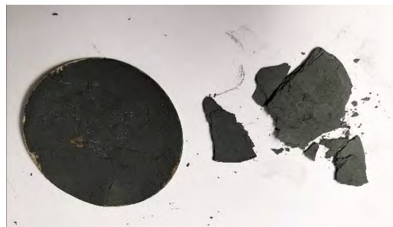
FIGURE 2. Ceramic hybrids cracked after further heat treatment at \approx 500 °C.
