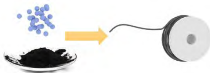
FIGURE 2. 3D-printable filaments made from the combination of ABS (blue beads) and Bosch carbon.
