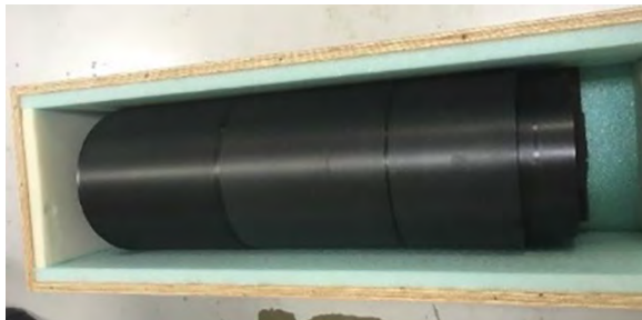
FIGURE 3. Three of four segments making up a full-scale fuel grain are shown being packaged for shipment.
