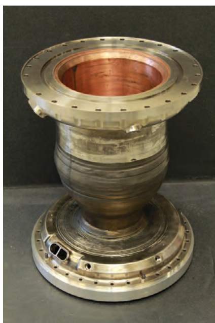
FIGURE 1. Combustion chamber showing the bimetallic bond of GRCop-84 liner and the Inconel 625 structural jacket and manifolds.
