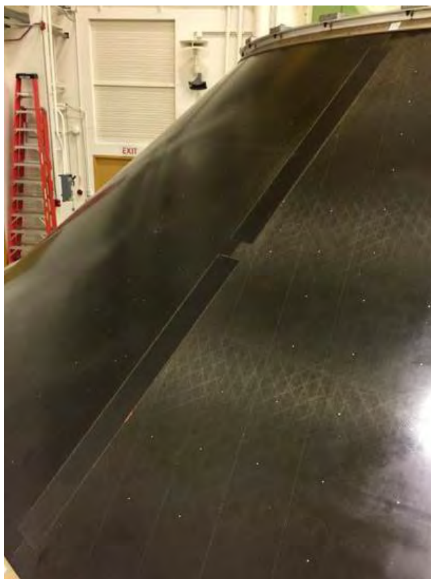
FIGURE 1. One of four full-scale bonded joints on the Payload Adapter Manufacturing Demonstration Article (PLA MDA).
