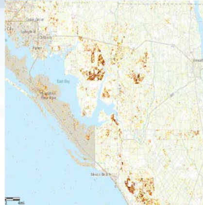
Damage Mapping: Damage proxy maps capture structure damage on immediate coastline
