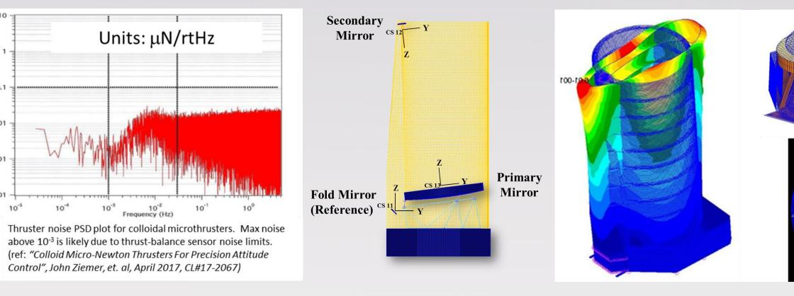
Predicted rigid body motion (with 4X MUF) caused by micro-thruster noise is several orders of magnitude below LOS Jitter Specification (left) and has margin against Primary Mirror Inertial WFE Specification (right). Actual micro-thruster performance is 2X lower than specification.
