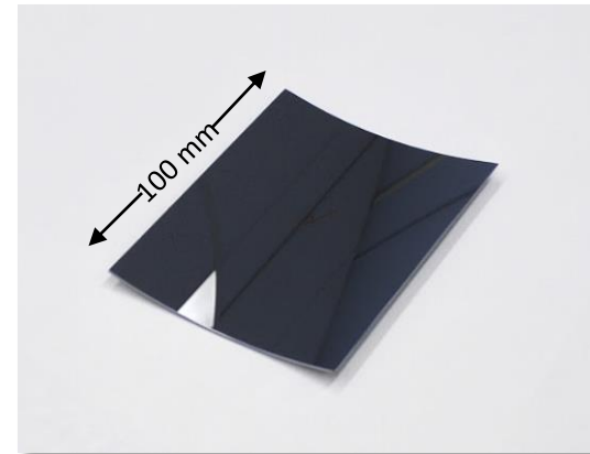
6. Trimmed mirror substrate
