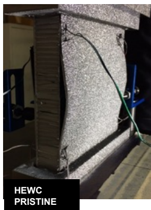
Failed HEWC Coupon
