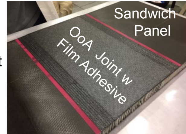
CTE Point Design Joint
