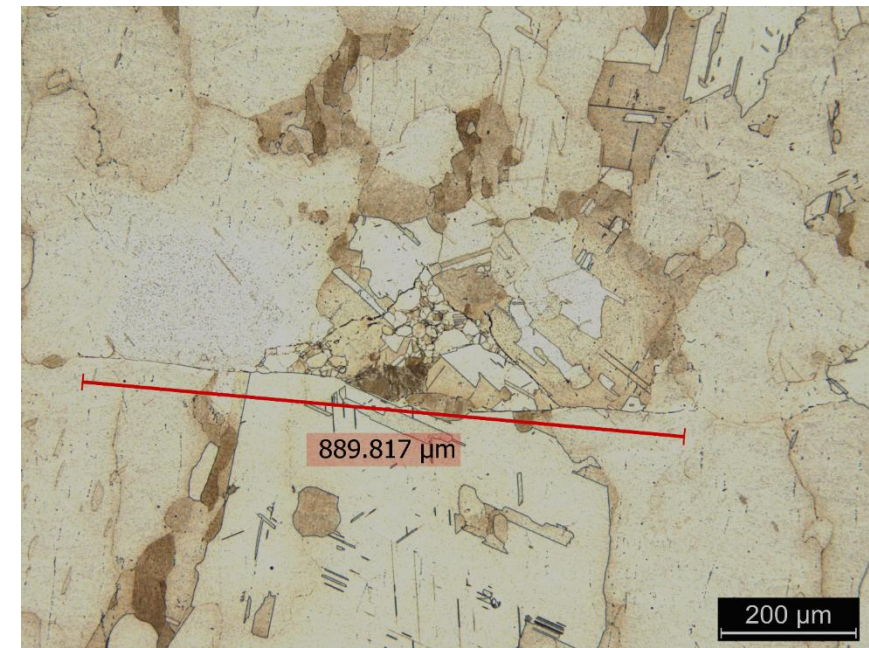
Lack of fusion defect after HIP
