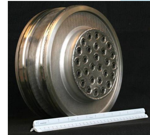
28-element Inconel ® 625 fuel injector built using an laser powder bed fusion (L-PBF) process
