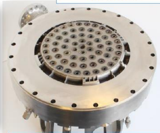
35K AMDE Injector with Welded Manifolds First Tested Nov 2015
