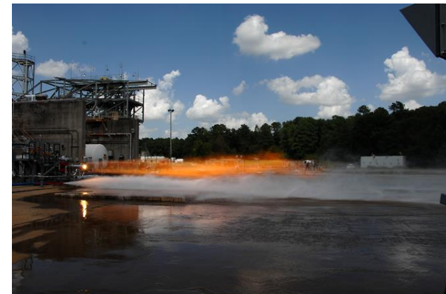
Hot fire test using L-PBF injectors
