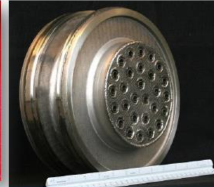
20K LPS Subscale Injector Tested Aug 2013 (3) Subscale Injectors Tested
