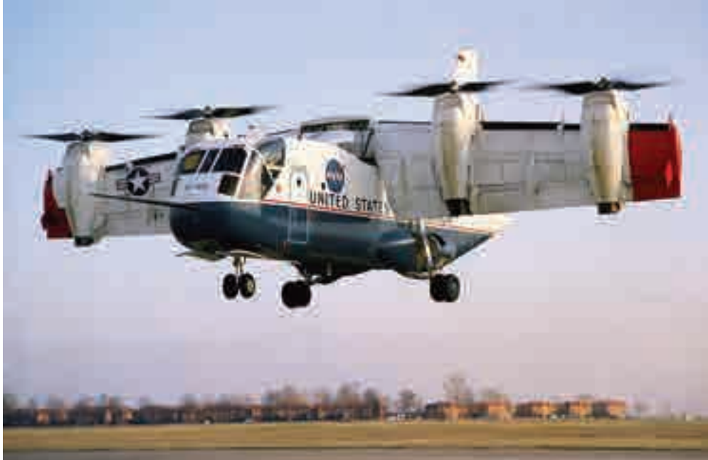
Fig. 2-76. The XC-142 tiltwing was built by Ling-Temco-Vought and Hiller and Ryan after they won the U.S. Air Force Tri-Service competition for an assault transport. The 41,500-pound aircraft, with a weight empty of 24,700 pounds, first flew on September 29, 1964.
