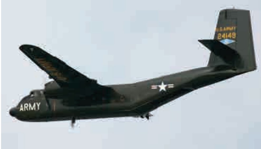
Fig. 3-164. The de Havilland DHC-4 Caribou made its first flight on July 30, 1958. This STOL aircraft became a favorite of the U.S. Army. However, in the mid 1960s, the U.S. Air Force took control of nearly all of the Army's fixed-wing machines. At a gross weight of 31,300 pounds and powered by P&W R2000 piston engines (1,450 bhp each), the Caribou could still operate out of 1,300-foot unprepared fields [495-498, 505, 604].
