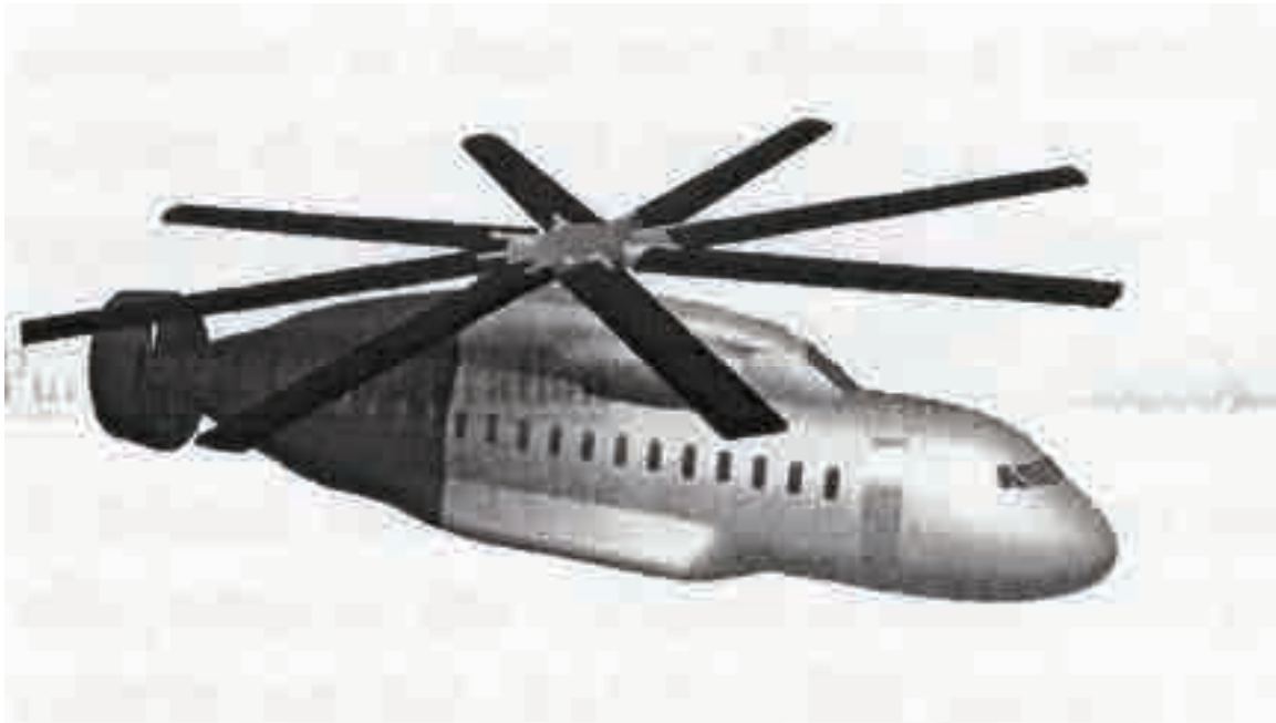
Fig. 2-199. Suppose you accept, say, eight blades attached to a hingeless hub, forget the wing, and operate the rotor at high speed at an advance ratio of 1.5 or higher. A Sikorsky paper [79] got me thinking.
