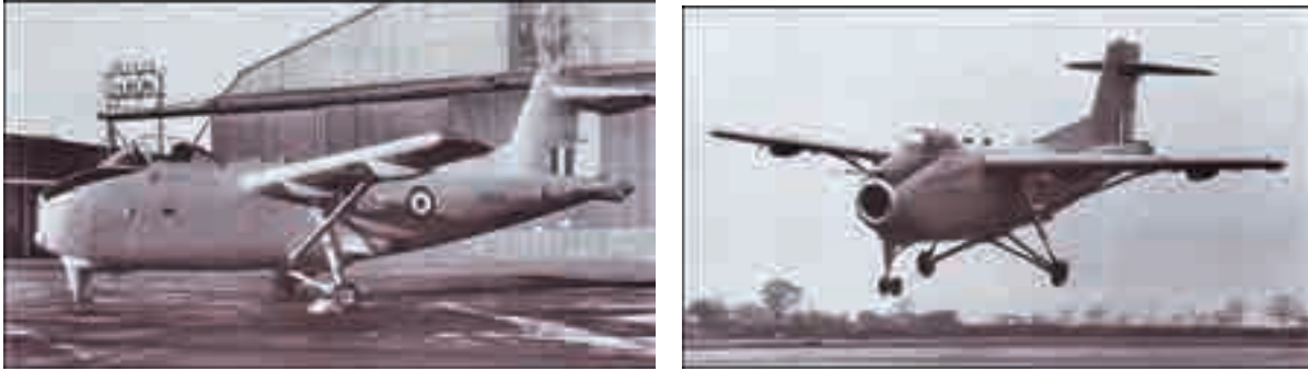
Fig. 3-53. The Hunting H.126 was a small, one-man British research demonstrator.
