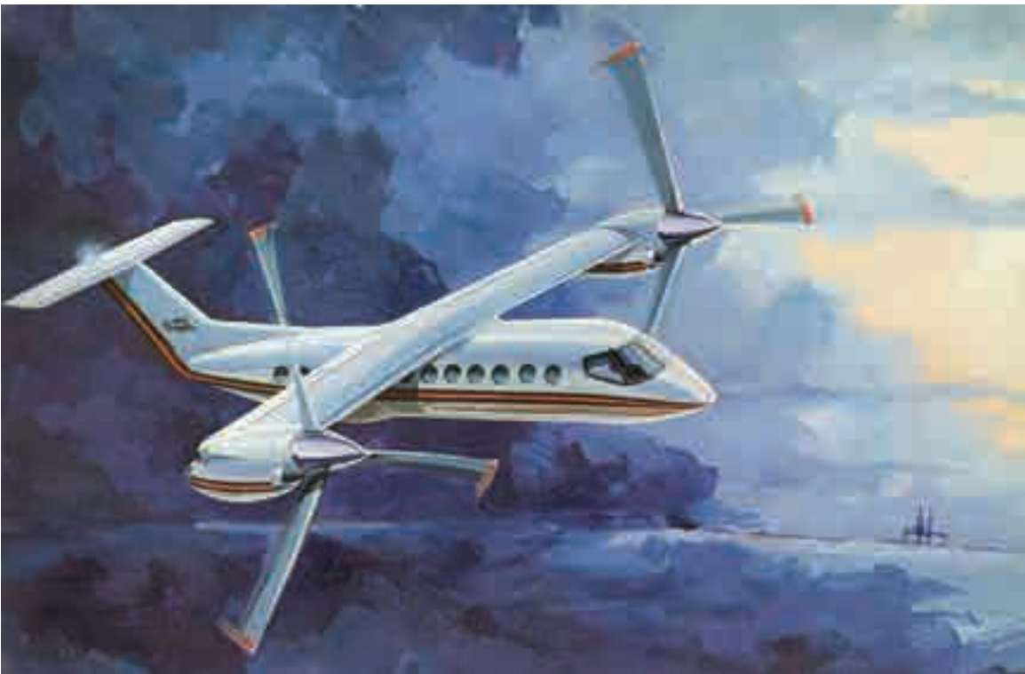
Fig. 2-190. Bell's D326 is a tiltrotor design that can compete with turboprop airplanes.
