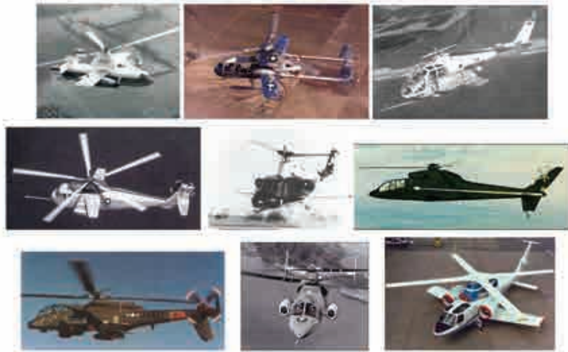
Fig. 2-44. Some past high-speed rotary wing aircraft (1950s through 1970s). Top row—Fairey Rotodyne, McDonnell XV-1, and Lockheed XH-51; center row—Sikorsky NH-3, Bell 533, and Sikorsky S-67; bottom row—Lockheed AH-56, Sikorsky S-69 Advancing Blade Concept, and Sikorsky/NASA/DARPA Rotor Systems Research Aircraft (RSRA) with a prototype x-wing installed (photos courtesy of Todd Quackenbush).
