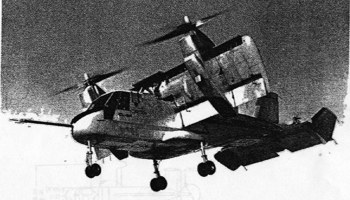
Fig. 2-89. Despite slats and flaps for stall mitigation, the Canadair CL-84 still had rates of descent limited to 700 feet per minute, which was well below operational requirements [210].
