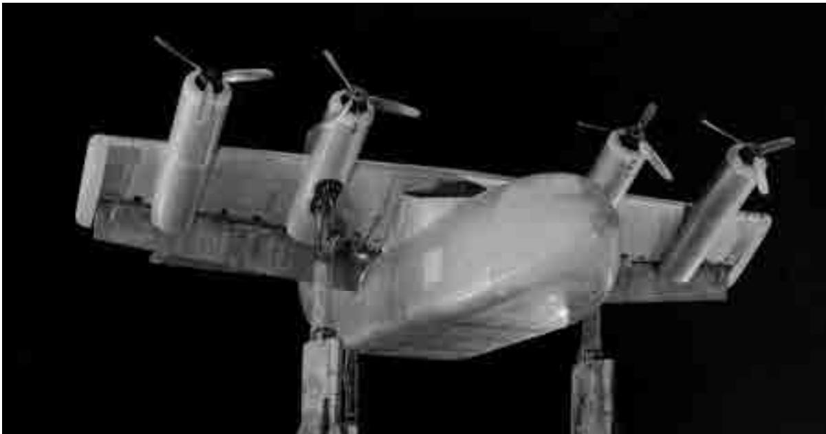
Fig. 3-103. The 0.4-scale model of the Fairchild C-123 after conversion to a severely cropped tiltwing (photo courtesy of Bill Warmbrodt, Ames Research Center).
