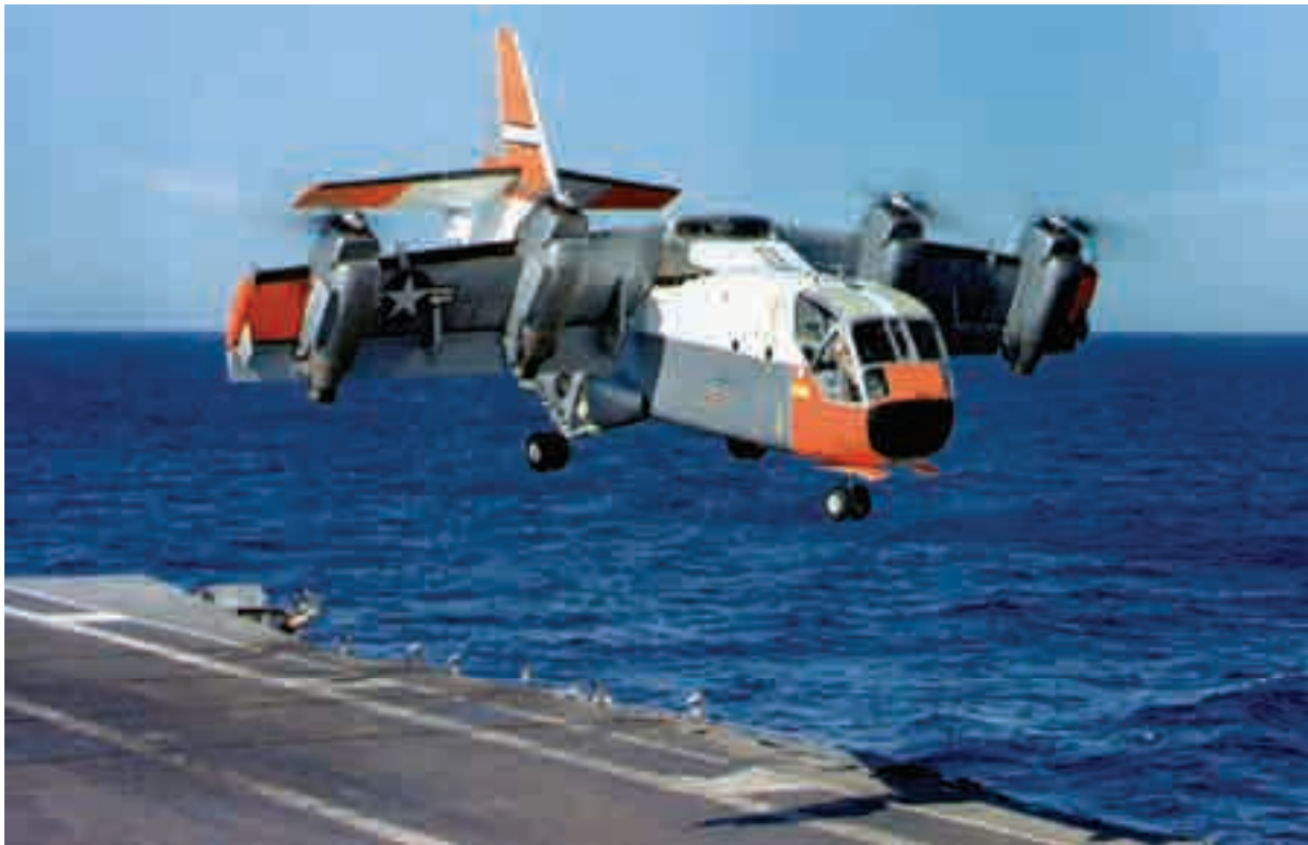
Fig. 2-105. The XC-142A had installed power for a maximum speed of 355 knots. This excess power equated to exceptional STOL performance. Navy sea trials were quite successful [39] (photo courtesy of Bill Norton).
