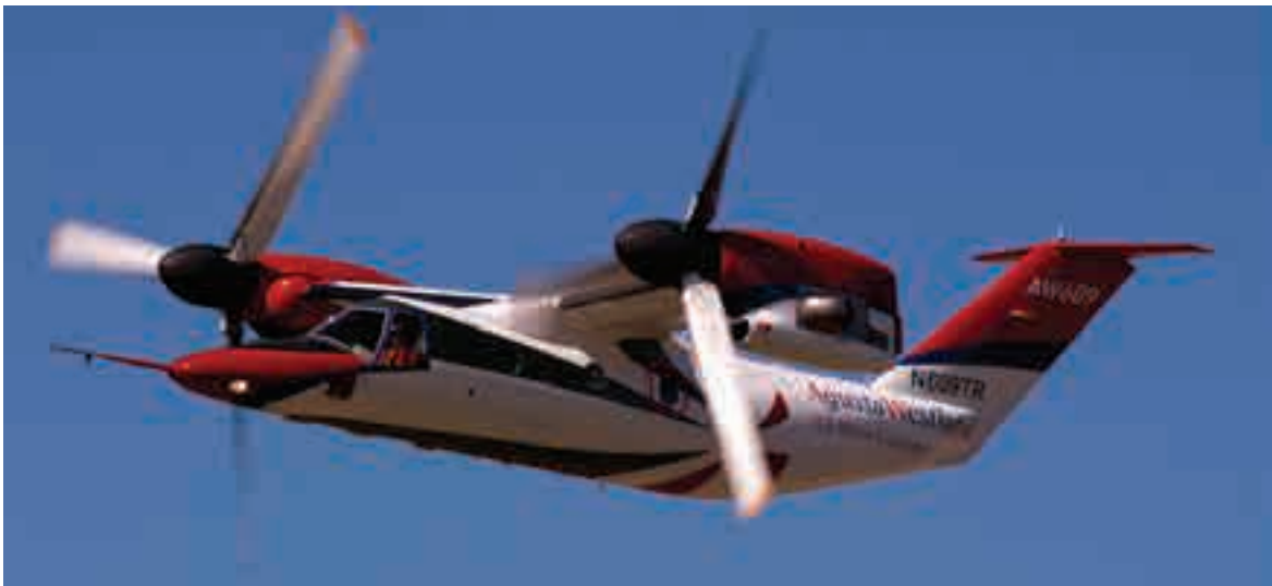
Fig. 2-196. The AW609 has a 16,800-pound VTOL design weight and a weight empty of 11,300 pounds. It is powered by two P&W PT6C-67A turboprop engines, each rated at 1,940 horsepower for takeoff at sea level standard day. It has demonstrated 333-knots maximum speed, and 275-knots maximum cruise speed. Note that the frontal area of the proprotor spinners and the nacelles behind appear nearly as large as the fuselage frontal area (photo courtesy of AgustaWestland).
