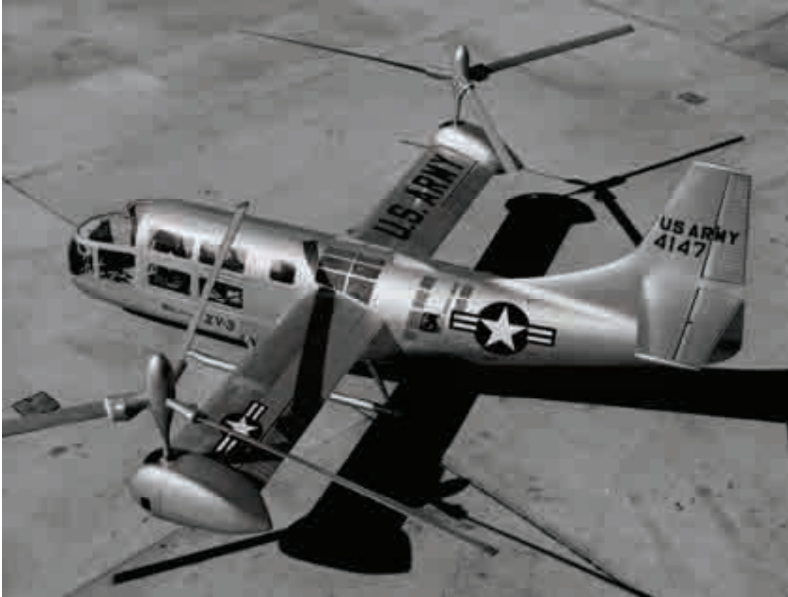
Fig. 2-125. The Bell XV-3 (s/n 54-4147) started out with three-bladed, articulated hinged rotors. A dynamic instability referred to as rotor-pylon instability, and later as whirl flutter, finally caused a catastrophic crash on October 25, 1956 (photo courtesy of Tommy Thomason).
