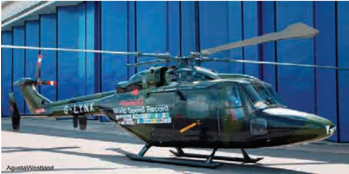
Fig. 2-49. The Westland Helicopter Limited G-Lynx set the current world speed record of 216.3 knots on August 11, 1986. The blade tips had a very tailored planform, commonly known as the British Experimental Rotor Programme (BERP) tip [143, 146].
