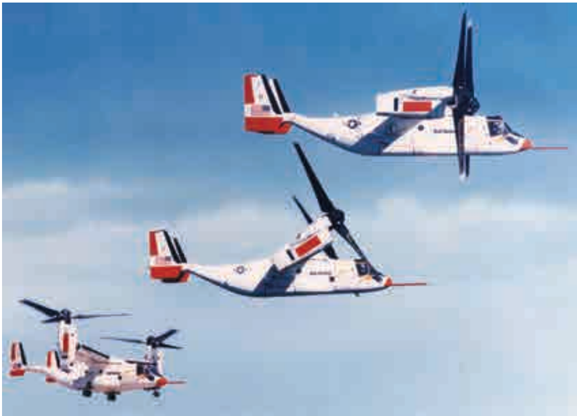
Fig. 2-63. The Bell/Boeing V-22 Osprey: a collage showing the aircraft in hover, then in transition with the rotors partially tilted, and finally in cruise flight.
