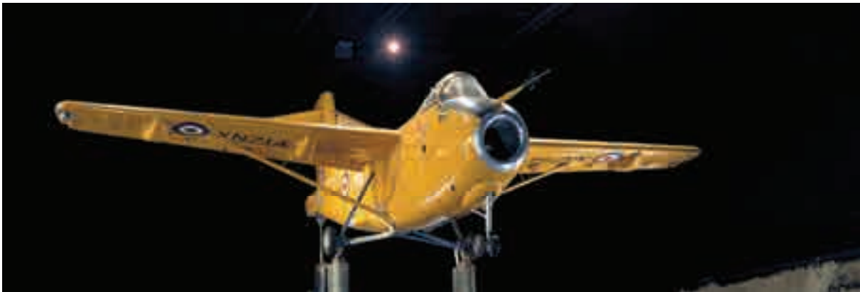
Fig. 3-54. The Hunting H.126 was tested in the NASA Ames 40- by 80-foot wind tunnel during June and July of 1969. The H.126 had a wingspan of 45.33 feet, a wing area of 221 square feet, and a wing aspect ratio of 9.3 (photo courtesy of Bill Warmbrodt, Ames Research Center).
