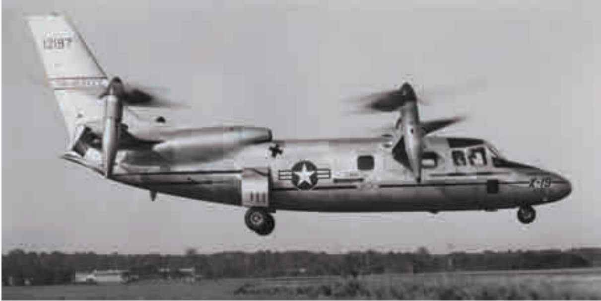
Fig. 2-95. The Curtiss-Wright X-19. This 10,600-pound VTOL technology demonstrator made its first hovering flight on May 7, 1965. The first full conversion back and forth from hover was made on January 17, 1968.
