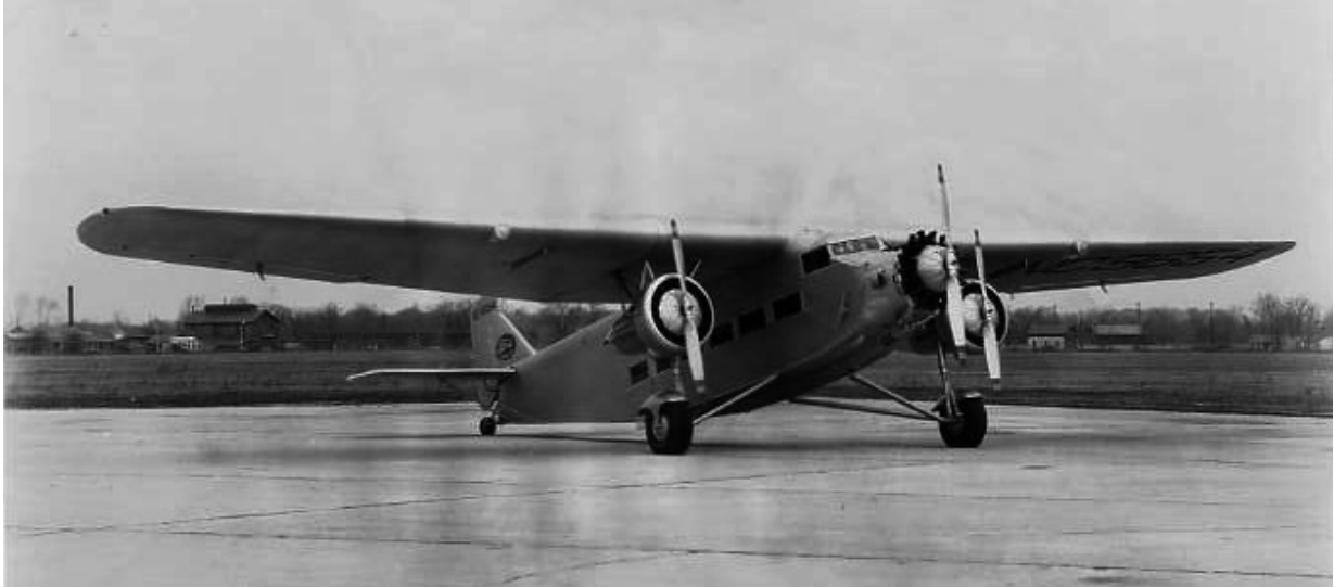
Fig. 3-200. The Ford Trimotor, a 12-passenger airliner, was developed by the Stout Metal Airplane Division of the Ford Motor Company. Its first flight was made on June 11, 1926. It did not, however, earn early airlines a profit. Still, the commercial airline industry expanded thanks to government subsidies.
