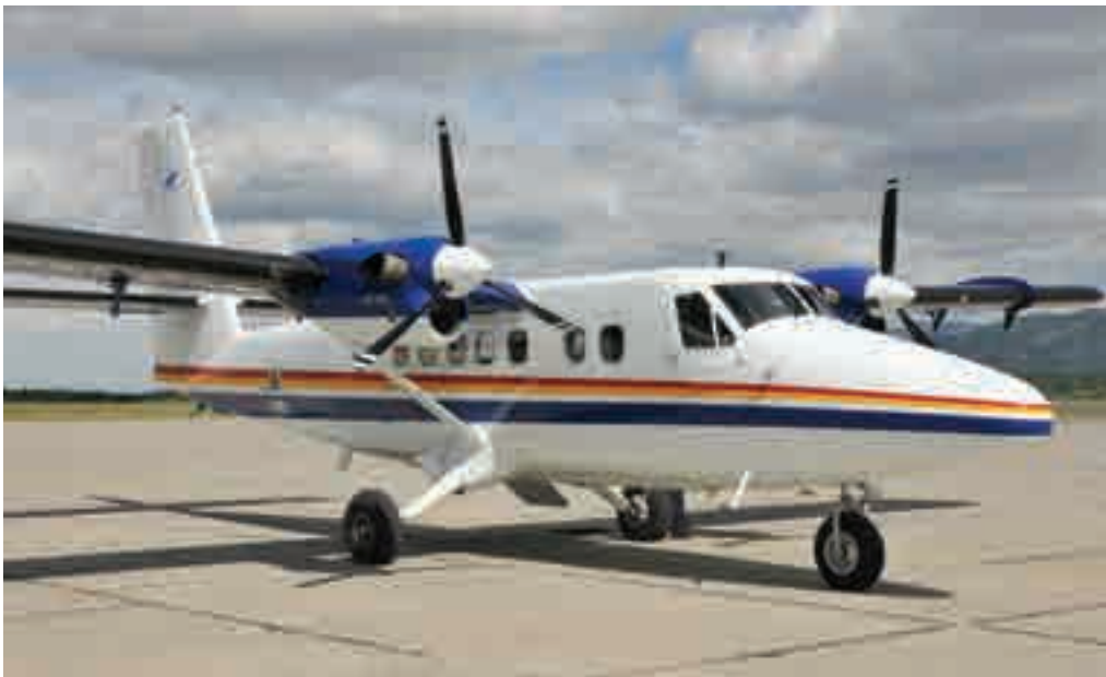
Fig. 3-163. The de Havilland DHC-6 Twin Otter first flew on May 20, 1965. This all-metal, 12,500-pound-gross-weight aircraft was powered by two P&W PT6A-27 turboprops, each having a 620 ESHP rating for takeoff. The Twin Otter continued de Havilland's design philosophy of 1,000-foot STOL performance. The rights to build the aircraft are now in the hands of Viking Air of Victoria, British Columbia [495, 507, 604].
