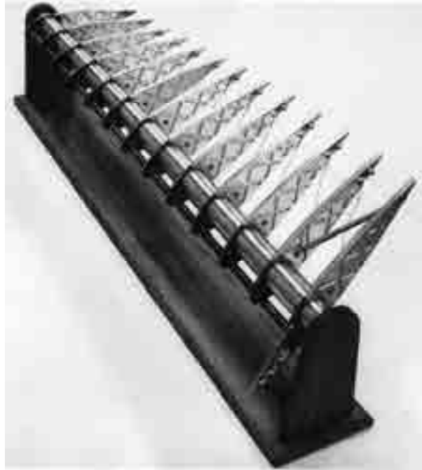
Fig. 2-9. The inboard segment of the twistable, segmented rotor concept as visualized in August of 1963 [92].
