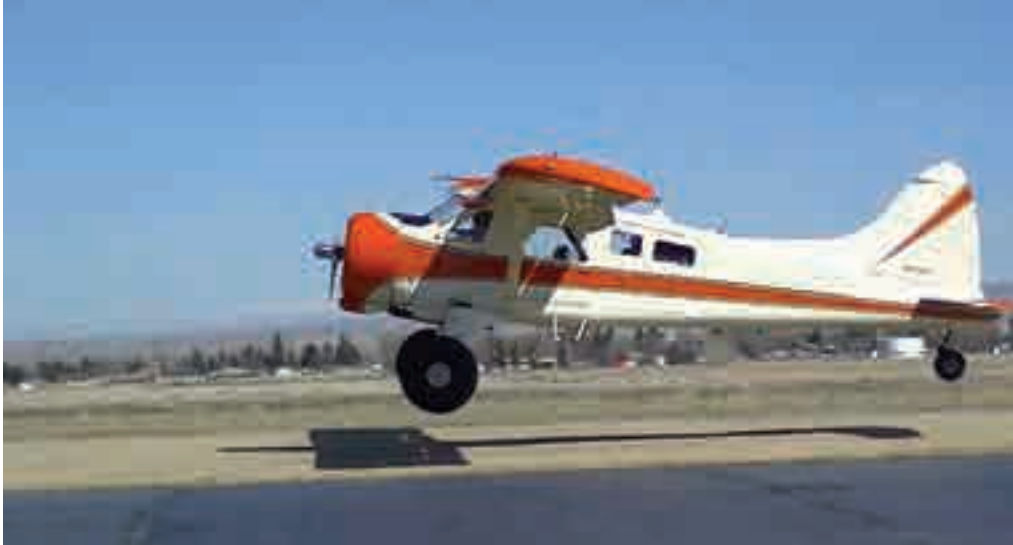
Fig. 3-160. The de Havilland DHC-2 Beaver established itself as a very rugged STOL for the backwoods. The aircraft was all metal. At its typical gross weight of 5,100 pounds, it could operate in and out of a 1,000-foot field surrounded by 50-foot obstacles. It was powered by a P&W 450 bhp R985 Wasp Jr. engine, and its first flight was August 16, 1947 [495, 503, 604].
