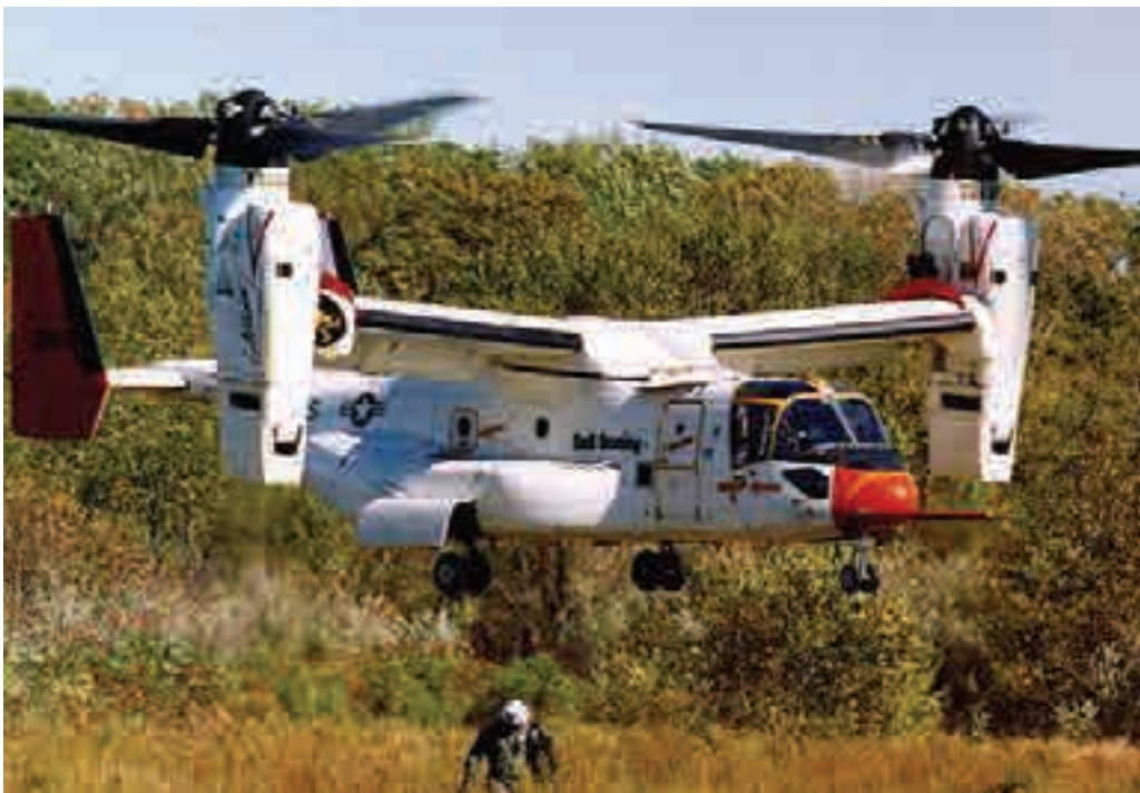
Fig. 2-77. The Bell Boeing V-22 tiltrotor is now in service with the U.S. Marines as an assault transport. This 52,600-pound aircraft, with a weight empty of 33,140 pounds, first flew on March 19, 1989.
