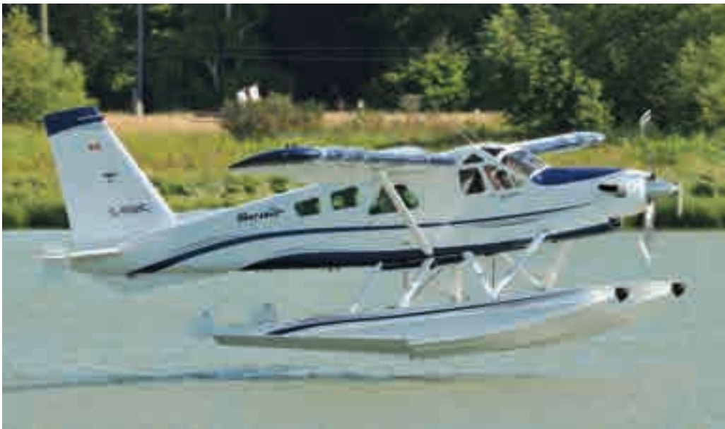
Fig. 3-161. The de Havilland DHC-2 Mk III Turbo Beaver was powered by a P&W PT6A-20, a turboprop engine rated at 550 ESHP. The takeoff gross weight was 5,370 pounds and the STOL performance was on par with the piston-engine-powered Beaver, while providing about a 200 pound increase in useful load. The aircraft could be flown with floats and skis as well as in land plane configuration [495, 604].
