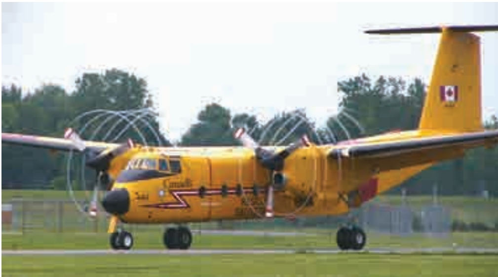
Fig. 3-165. The de Havilland of Canada CC-115 or the U.S. Army CV-7A Buffalo [477, 478, 495, 499, 506, 604]. The maximum STOL takeoff gross weight was 49,200 pounds, which put it in competition with the Air Force Fairchild C-123B. The Buffalo was powered by two turboshaft CT64-820-4 General Electric engines, each with a takeoff rating of 3,133 ESHP. The three-bladed, 14.5-foot-diameter propellers were Hamilton Standard (model 63E60-13) and normally operated at 1,160 rpm. Of course, the U.S. Army Buffalo became U.S. Air Force property in the roles and mission settlements and was redesignated as the C-8.
