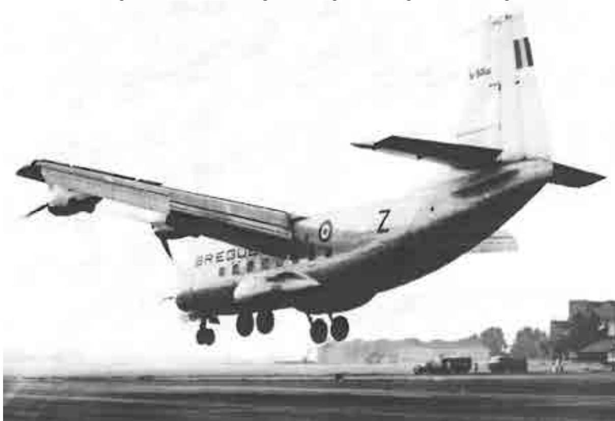
Fig. 3-112. The four propellers were interconnected on the Bréguet 941 because of success demonstrated by the smaller Bréguet 940 (photo courtesy of Bill Warmbrodt, Ames Research Center).
