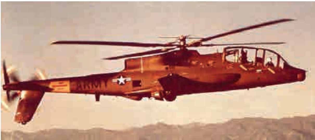
Fig. 2-46. The AH-56 rotor reached an advance ratio slightly over 0.52 at a flight speed of 204 knots.
