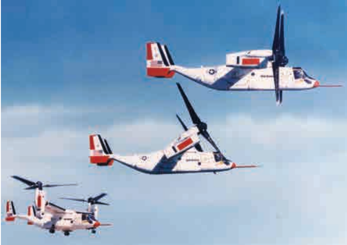
Fig. 1-23. The Bell/Boeing V-22, a VTOL transport powered with gas turbines. A collage showing the aircraft in hover, in transition with the rotors partially tilted, and in cruise flight.
