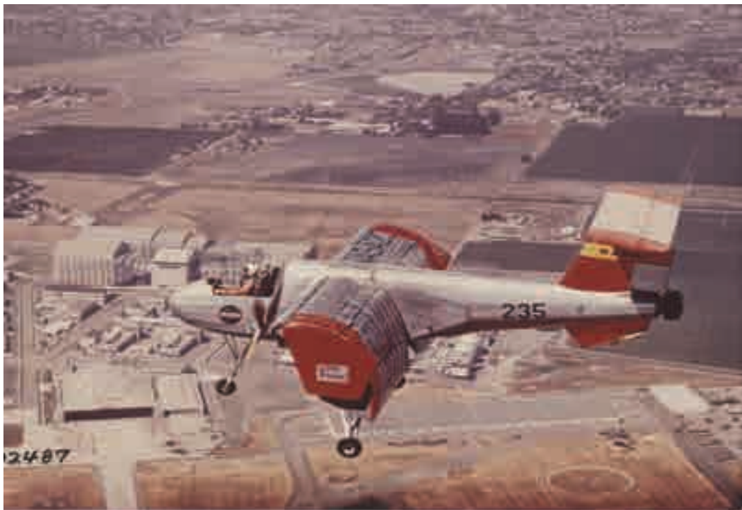
Fig. 3-95. The Ryan VZ-3, along with several NASA wind tunnel experiments, established what potential the deflected slipstream concept had for VTOL. The wingspan was 23 feet and the gross weight was about 2,600 pounds. The general conclusion was that the approach was not too promising, and now the aircraft is on display at the U.S. Army Aviation Museum in Ft. Rucker, Alabama.
