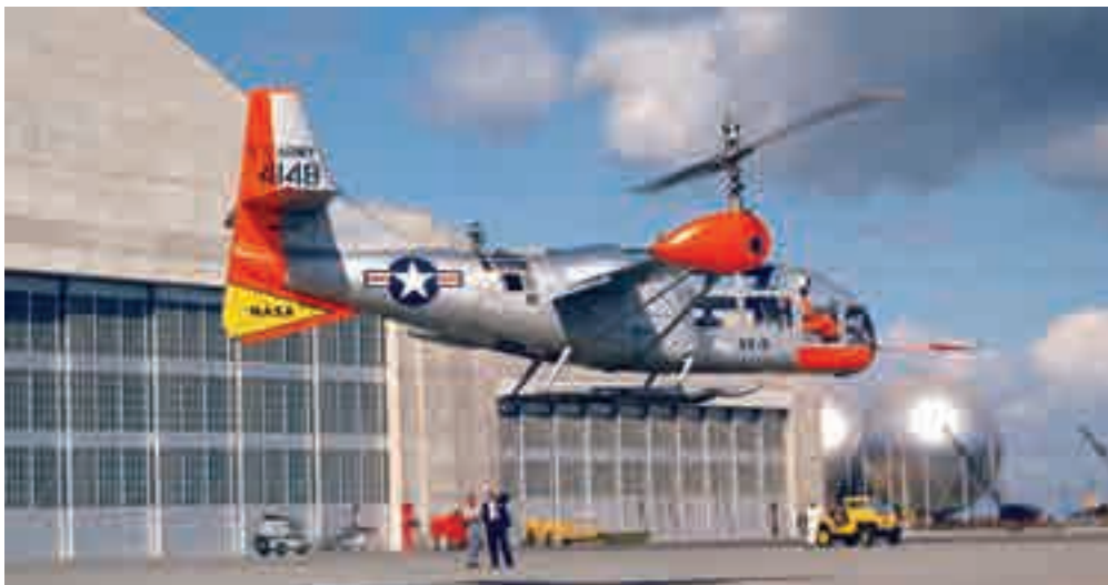
Fig. 2-126. The XV-3 (s/n 54-4148), the second aircraft, used Bell's "standard" two-bladed, teetering rotor, which, along with several other fixes, suppressed whirl flutter enough that military flight test evaluation could be completed [256].
