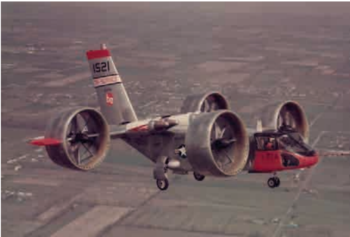
Fig. 2-96. The Bell Aerospace X-22A. This 15,300-pound VTOL technology demonstrator made its first hovering flight on March 17, 1966. The first full conversion back and forth from hover was made on March 3, 1967.
