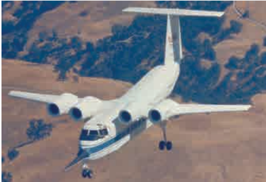
Fig. 3-196. NASA's QSRA, a Boeing conversion of a de Havilland Buffalo, first flew July 6, 1978. Operational weight empty was 36,800 pounds; normal takeoff weight was 50,000 pounds. Wingspan was 73.5 feet with an area of 600 square feet. Each Avco YF102 turbofan engine was rated at 7,500 pounds thrust [641-646].
