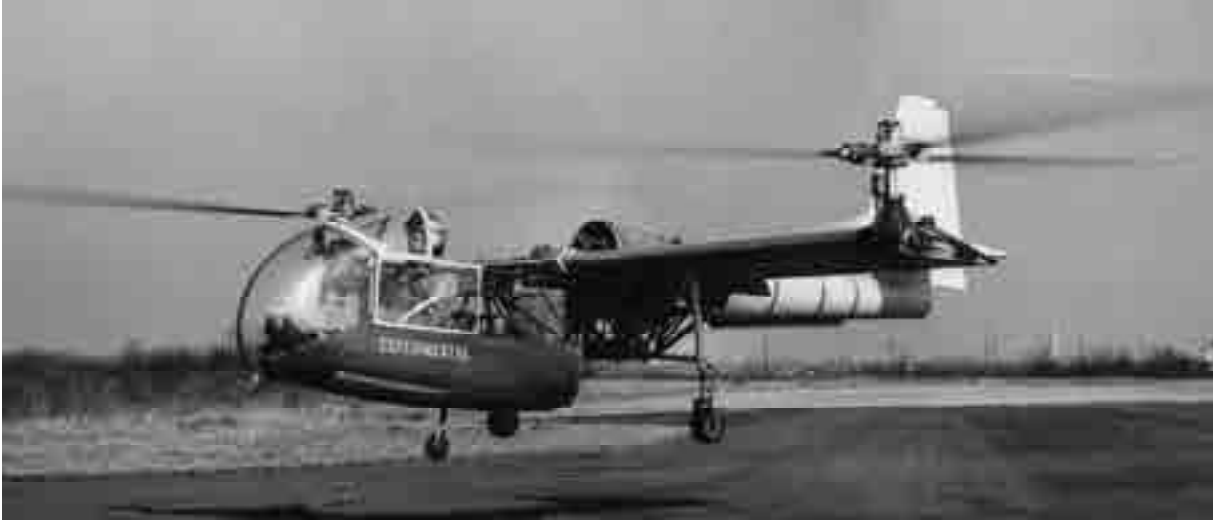
Fig. 2-119. The Transcendental Model 1-G. This 1,750-pound VTOL technology demonstrator made its first, untethered, hovering flight on July 6, 1954. The preceding Model 1 was destroyed by ground resonance. This classical, early autogyro and helicopter mechanical instability problem was overcome with the Model 1-G. Only partial conversions from a shaft tilt of 0 degrees (hover) to about 70 degrees forward (airplane) were completed. On July 20, 1955, during a test flight in which the conversion was virtually complete, the aircraft dove, nose first, into the Delaware River (photo courtesy of Howard Levy and Mike Hirschberg).
