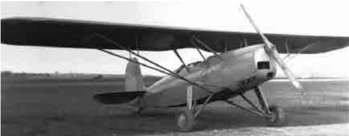
Fig. 1-6. The Fairchild 22 C7 had a 75-hp engine. The wingspan was 32.83 feet with a 66-inch chord and an area of 170 square feet. The weight empty was 870 pounds, and the gross weight was 1,400 pounds. It sold for $2,675 at the factory [10].
