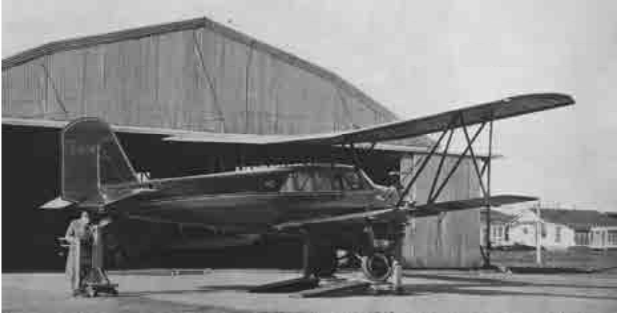
Fig. 1-1. The Glenn Curtiss Tanager was the outright winner of the Guggenheim Safe Aircraft Competition. It featured manually controlled flaps, floating ailerons, long-stroke rugged landing gear, and independently operated brakes.
