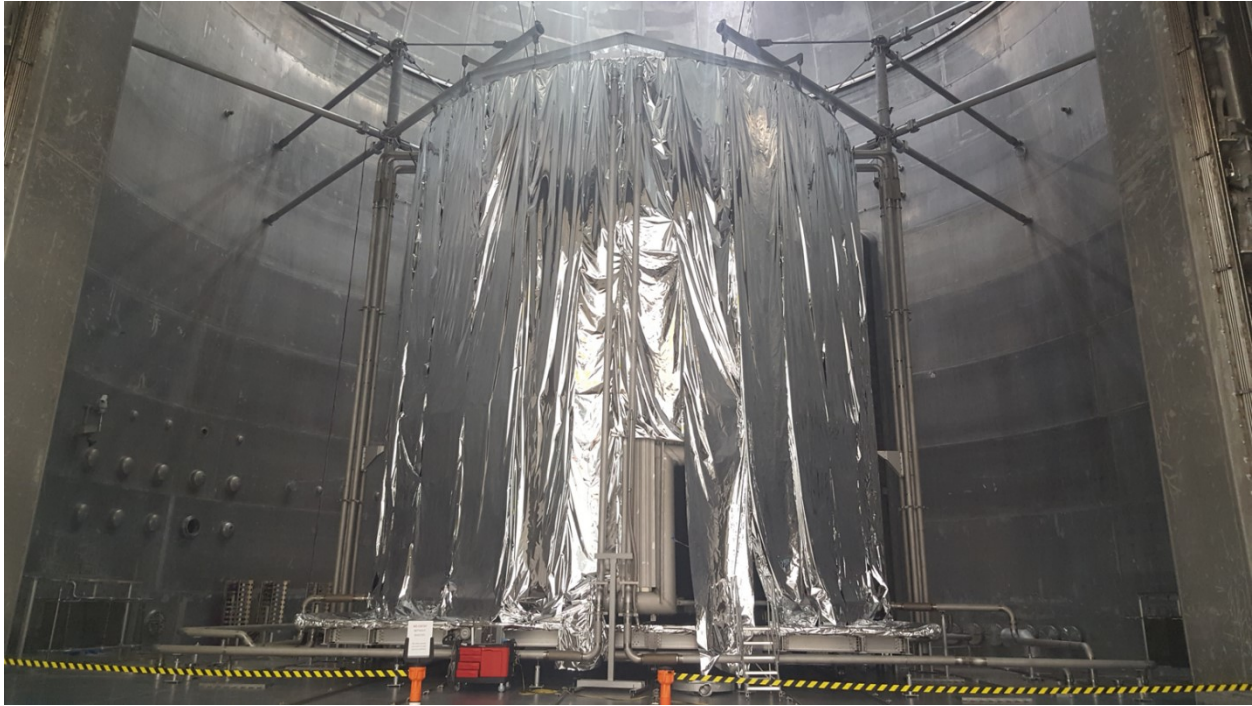
Figure 9. Vacuum chamber and cryoshroud prior to bake-out.
