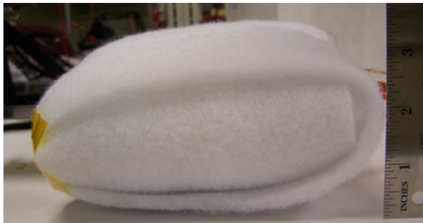
Figure 14.—Side view of insulation surrounding heat pipe 2 evaporator.
