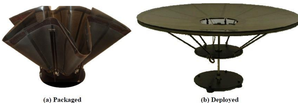
Figure 18 Flexible precision reflector before and after deployment [26].
