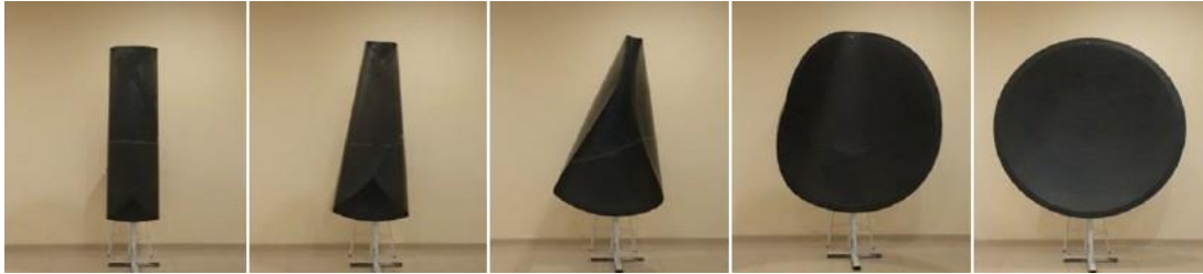
Figure 19 Deployment of the self-deployable shell reflector (duration: 1.4 s) [28].
