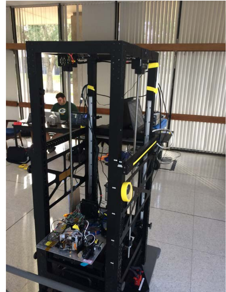
Seeker FlatSat on ROSIE Platform for HSI-3
