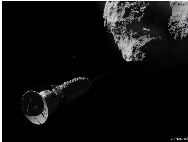
Figure 52: Concept drawing of a Comet Hitchhiker spacecraft, performing a hitchhiker maneuver at a small body in the outer Solar System.
