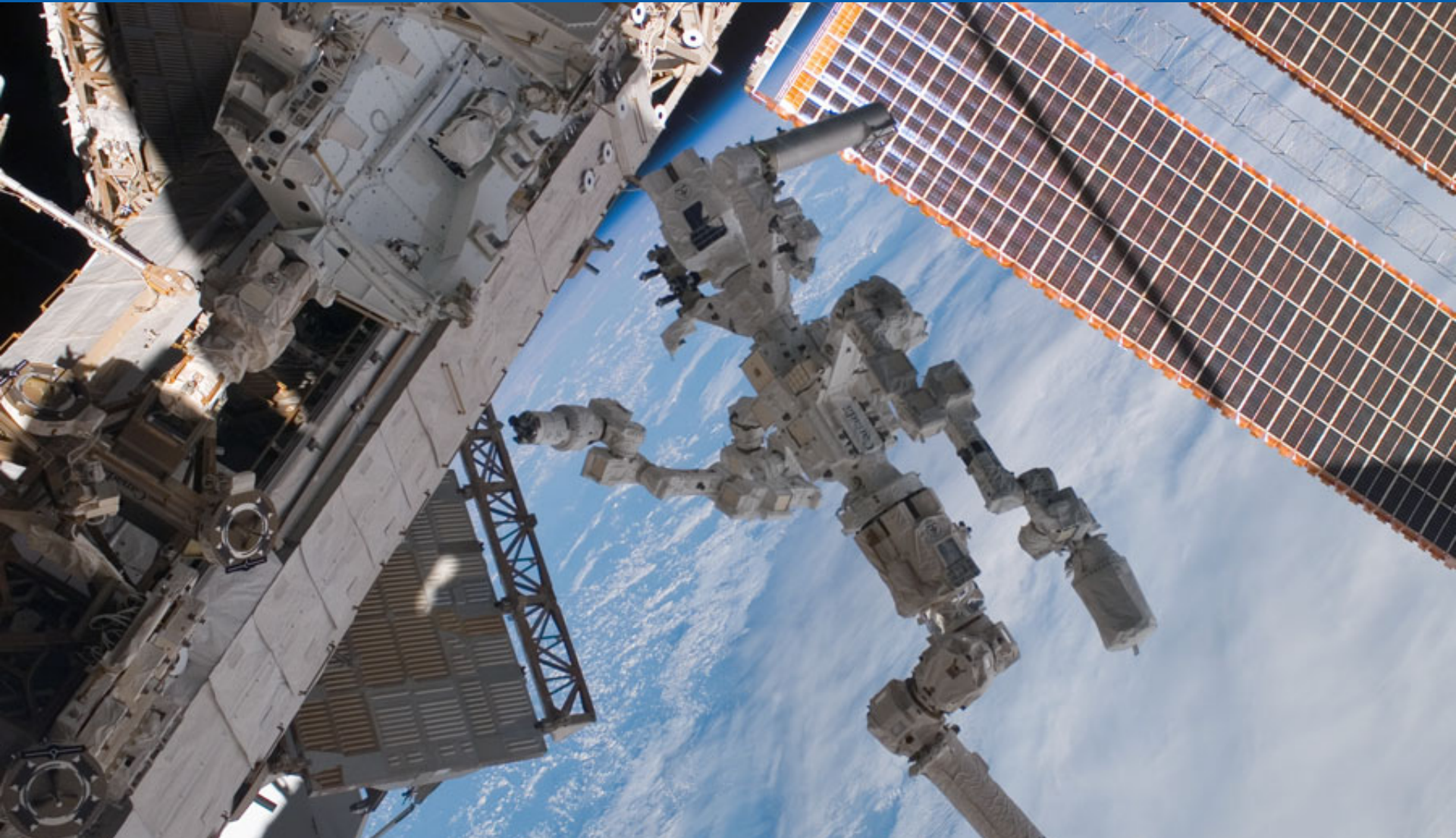
Special Purpose Dexterous Manipulator (“Dextre”)
