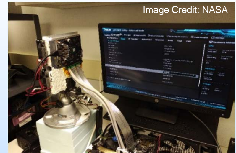
400 W cooling on bare NVIDIA GTX 1050 E. Wyrwas, 2018 NEPP GPU BOK .
