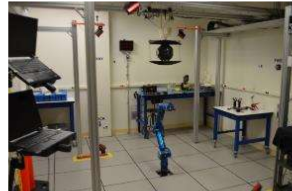
Micro Gravity Test Facility (MGTF) Lab: Cradle/Gimbal and Robotic ARM
