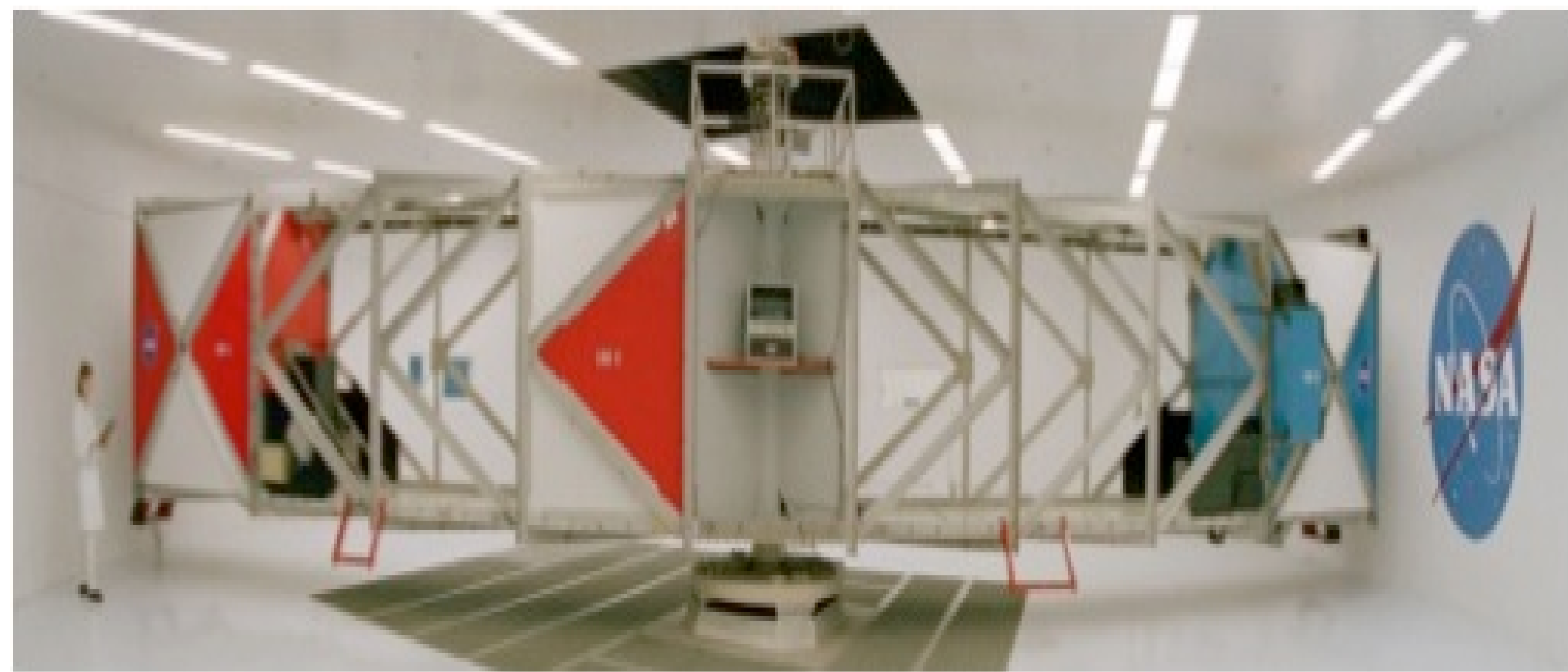
20-G Human Centrifuge, ARC, Moffett Field, CA. Use for pre-flight ground study and live return Ground Controls in the future.
