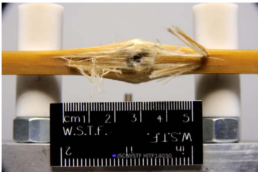
Figure 32: Front Close-up View of ISS SAW Mast Degradation Flex Batten Test #1
