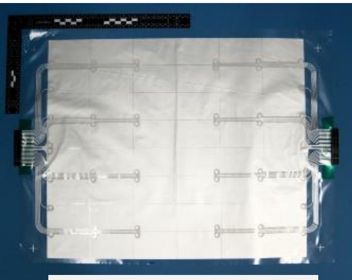
Piezoelectric impact sensor film (18" x 16", with 48 pixels)
