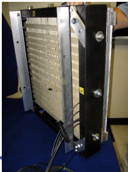
Test article (2'x2') with integrated sensors & piezoelectric sensor array
