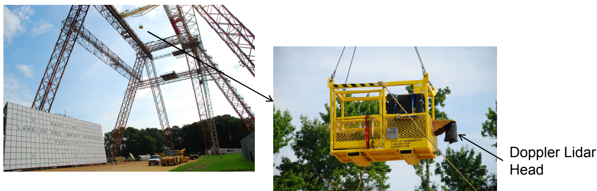
Figure 24. NDL system dynamic testing at NASA LaRC Gantry
