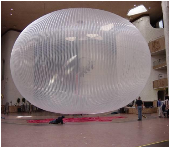
Figure 8: Example of an inflatable that uses the “gore” fabrication technique.
