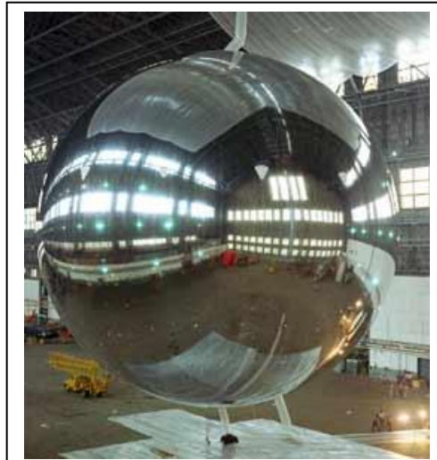
Figure 3: Pageos 1 Satellite during tests in 1965: 30.5 m in diameter, 0.5 mil Mylar.
