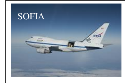
Figure 17: Top: JWST is the NASA flagship IR/FIR mission with a 6.5 m telescope for >$5B. Middle: SOFIA is a 2.5 m airborne IR/FIR telescope for >$1B. LBR is a 10 m FIR/THz sub-orbital telescope for <$0.01B.
