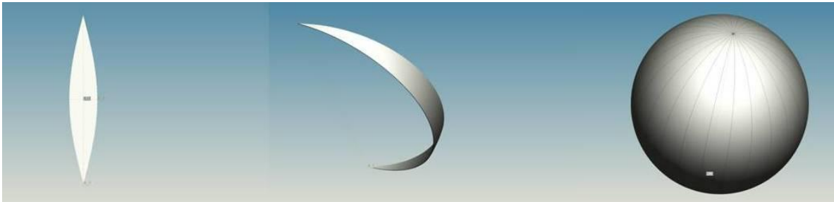
Figure 7: Typical “gore” pattern sections used in most scientific balloons
